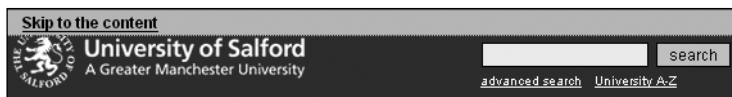
Figure 15-17. New skip to the content link, now also visible to sighted keyboard users
