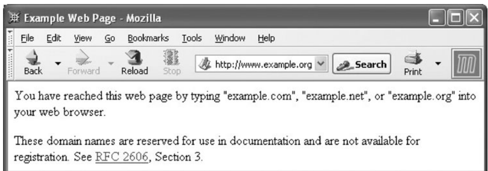
FIGURE 1.3 Web browser displaying information received in an HTTP response message received after the browser sent an HTTP request message to a web server. The content shown is subject to copyright and used by permission of the Internet Assigned Numbers Authority (IANA).
