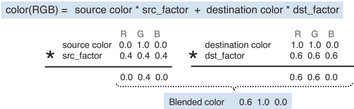
Figure 10.14 Calculation of gl.blendFunc(gl.SRC_ALPHA, gl.ONE_MINUS_SRC_ALPHA)
