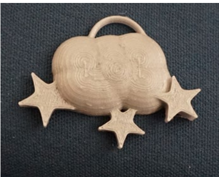
Figure 10-6. The clouds and stars print close up—compare with Figure 10-3 preview
