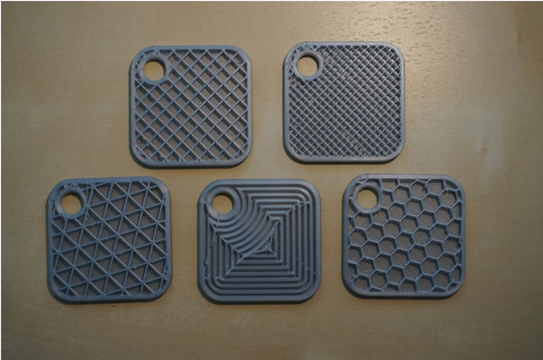
Figure 5-10. Different types of infill available from MatterSlice: Top—Grid (R) and Lines (L). Bottom—Triangles (L), Concentric (middle), Hexagon (R)
