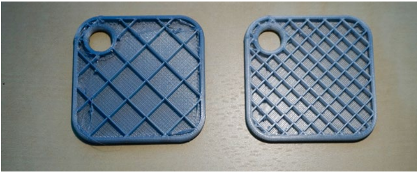
Figure 5-12. 10% and 25% MatterSlice infill patterns
