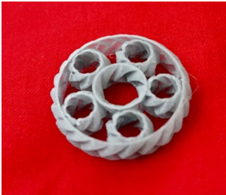
Figure 10-17. The resulting print of Rich's gear bearing. Note how thin the walls are
