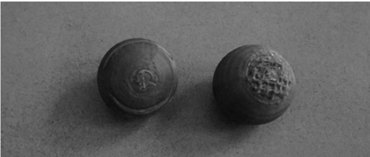
Figure 10-12. Completed somewhat cleaned-up spheres, without support (L) and with (R)
