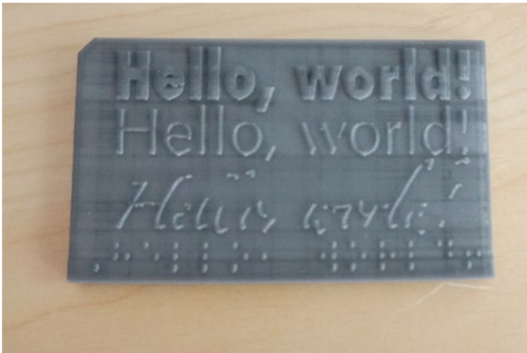
Figure 10-15. Closeup of the vertically printed (one side on the platform when printed) protruding text block
