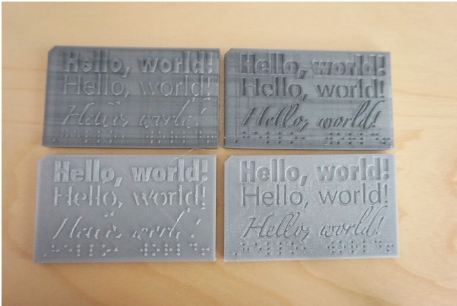
Figure 10-14. As-printed four blocks. Top two were printed with the surface vertical; the bottom two were printed flat on the platform. Protruding text is on the left, recessed on the right
