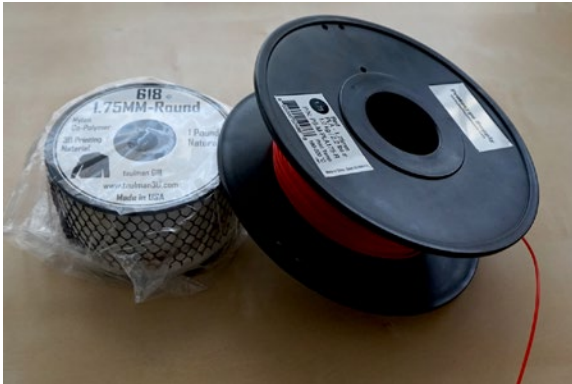
Figure 7-1. Typical spools of nylon (L) and PLA (R) filament
