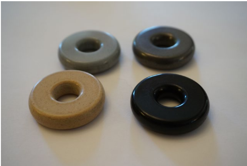
Figure 12-8. Four pieces that Rich printed and hand-sanded. Top left and front right are PLA. Top right is metal-filled PLA; lower left is wood-filled PLA
