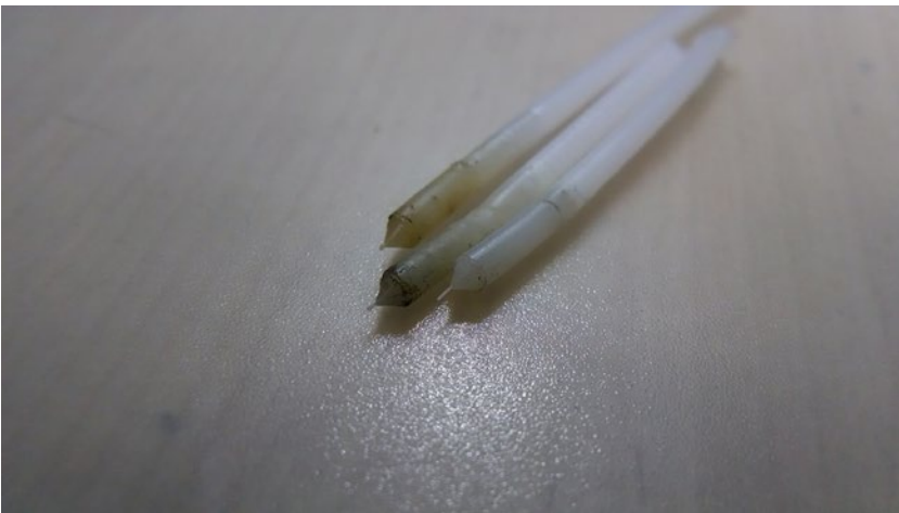
Figure 12-3. Nylon with residue of overheated plastic
