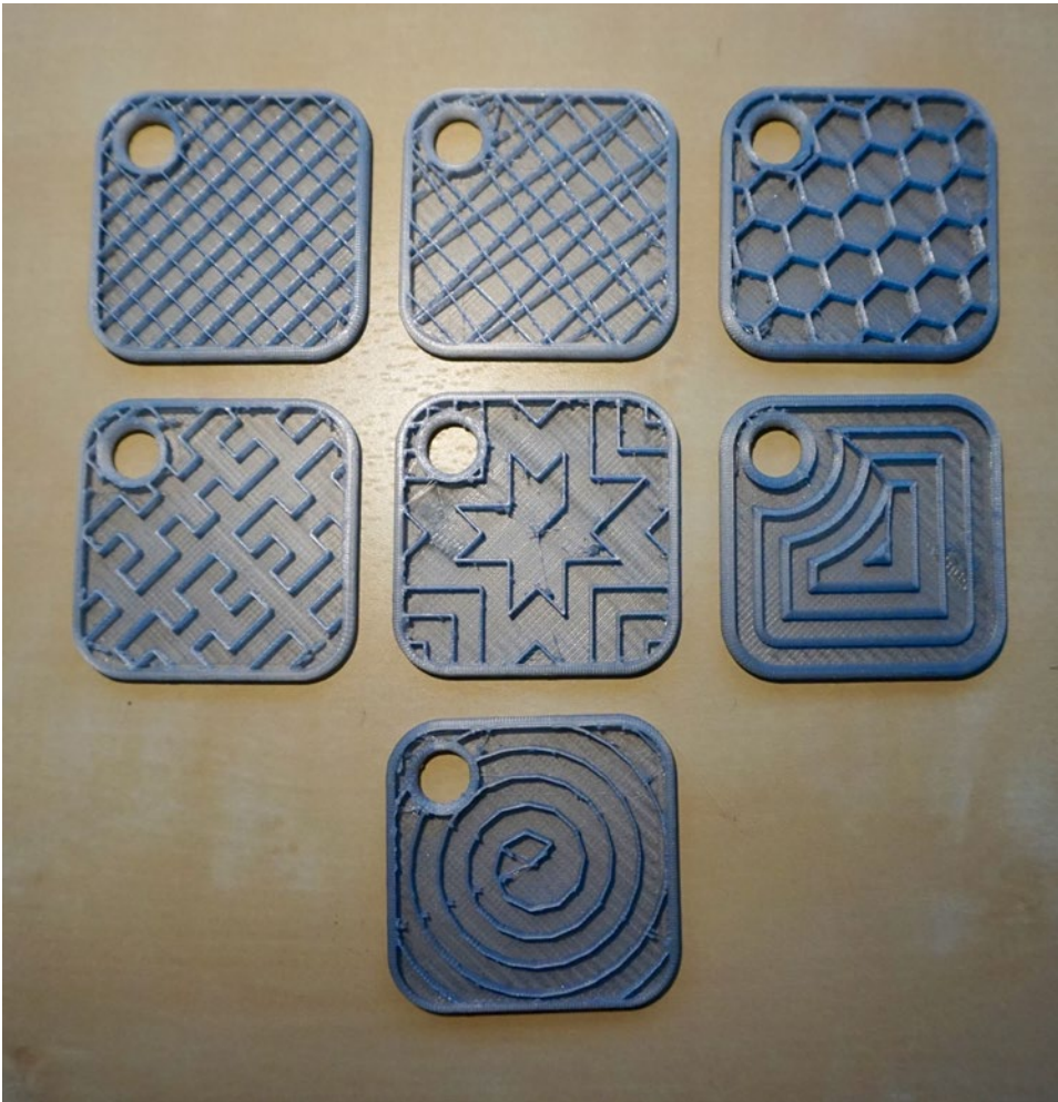
Figure 5-11. Different types of infill available from MatterControl Slic3r: Top row, L-R—rectilinear, line, honeycomb. Middle row—hilbertcurve, octagramspiral, concentric. Bottom row—archimedean chords
