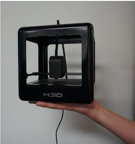
Figure 1-3. A Cartesian 3D printer with a direct-drive extruder (M3D)
