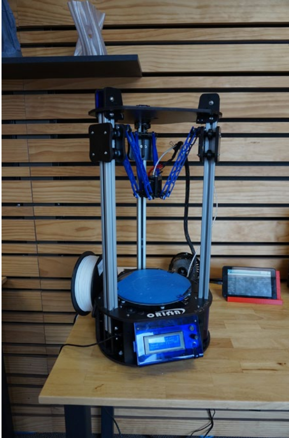
Figure 1-5. A deltabot (Orion by SeeMeCNC)
