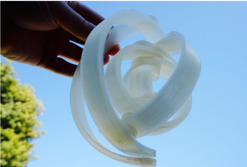
Figure 12-10. The same piece as in Figure 12-9, but in motion. This also shows how translucent natural (undyed) PLA can be
