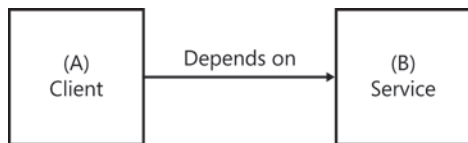
FIGURE 2-1 In any dependency relationship, the dependent is referred to as the client , and the entity that is being depended on is the service .
