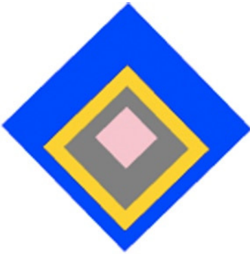
Figure 4-4. If you rotate a parent, its children match its axis of rotation
