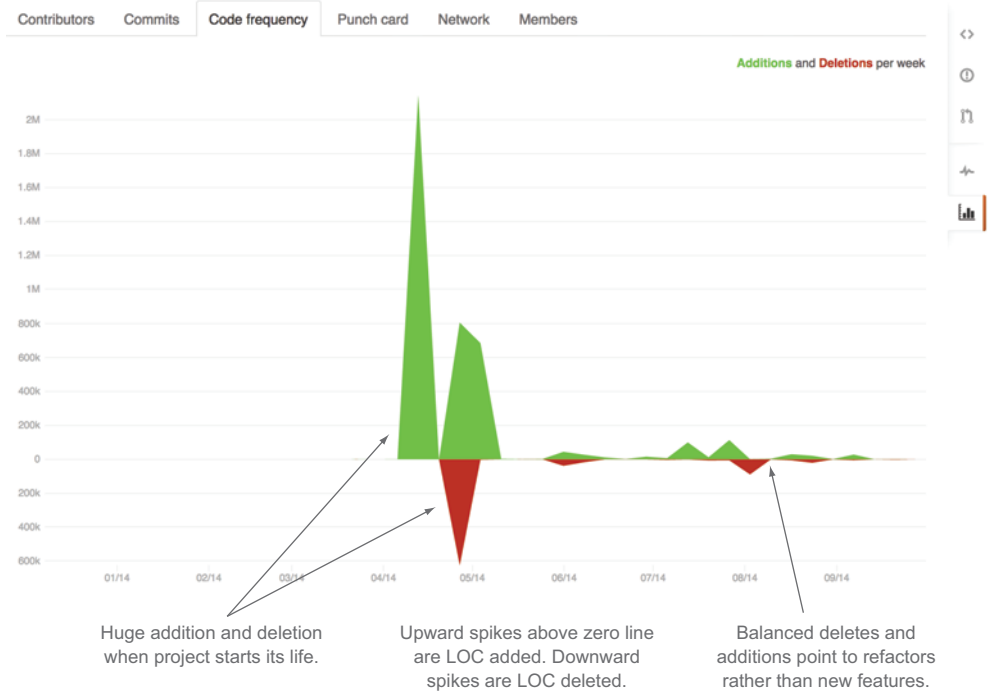
Figure 4.13 The Code Frequency tab shows how much code is changing over time in CLOC. From GoCD ( github.com/gocd/gocd/graphs/code-frequency ).
