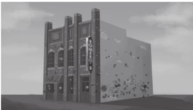
FIGURE 2.25 This perspective sketch of a building was painted over a simple 3D rendering. Such underlays can be used to create multiple looks for the same model.
