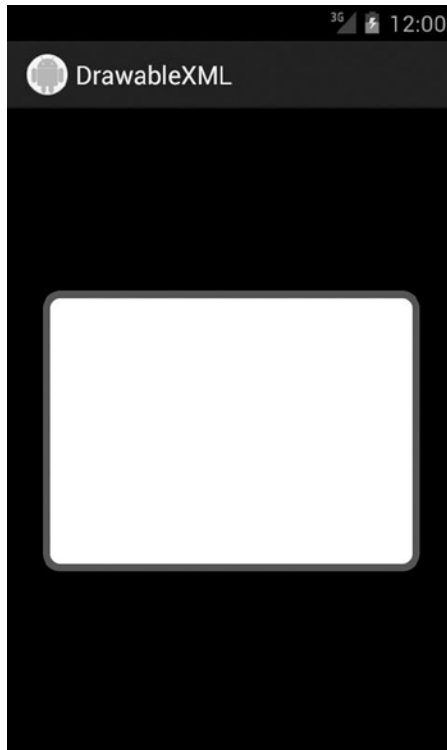
Figure 7-2. Rounded rectangle with border as view background
