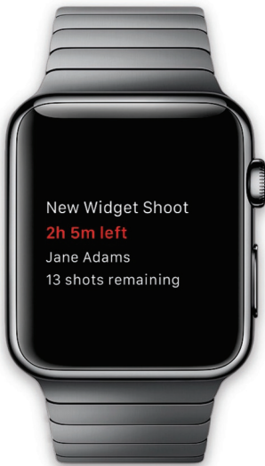
Figure 3.35. Simple UI that answers the questions of why, when, who, and what for a photographer that is on location at a shoot
