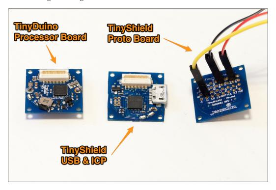
Of course, you can use any other small Arduino boards such as Arduino Micro. You can also use an Arduino Mini for this project. Any basic Arduino board that will fit into the device you want to hack will work.
