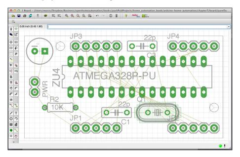
I then used the auto-routing function of EAGLE to automatically connect all the components on the board according to the schematic, as shown in the following screenshot:
