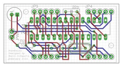
You can see that the Arduino controller is located in the middle of the board, surrounded by the IO pins and components that are necessary for the Arduino operation.
