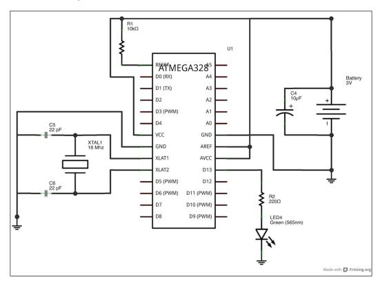
I recommend putting the Arduino microcontroller (ATmega328) first in the middle of the breadboard so you can add the different components around it. This schematic illustrates the placement of the different components:
