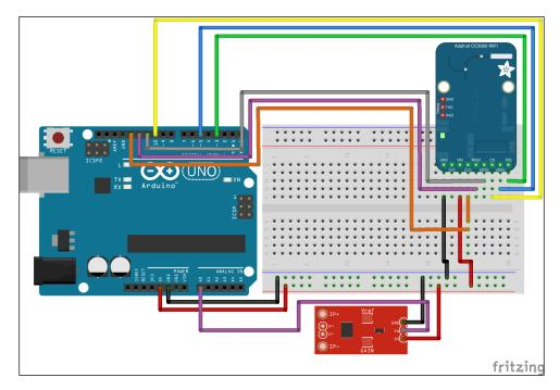
Now, you can connect the power cables to the current sensor so you can connect a device to the system:
