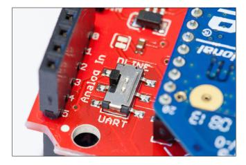
You will also need to connect the XBee explorer board to your computer at this point. Simply insert one XBee module to the board as shown in the following image:
