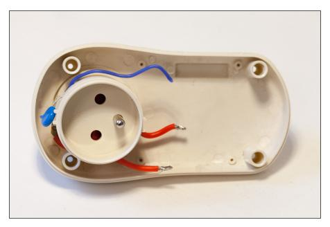
These two cables will have to be connected together if we want to get some current to flow into the device that is plugged into the hacked device. To do so and control the plug from the Arduino board, you need to insert the relay module now.
