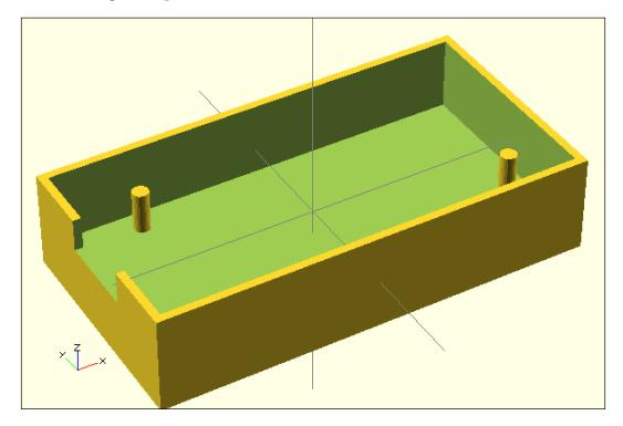
I also designed a cover to be able to close the case using the same principles. It is based on the union of two cube objects, so it fits nicely in the main part of the case.
