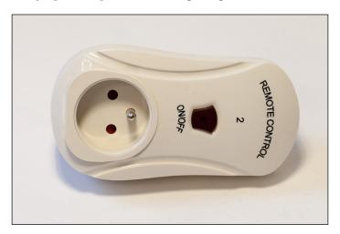
You can take any similar device, the most important thing being that the device is somehow controllable from an electronic system such as a remote control. This is important as we will later insert a relay inside the enclosure to control the switch. Mechanical controllable switches (for example, with only an on/off button on it and no electronics inside) won't work for this project.
