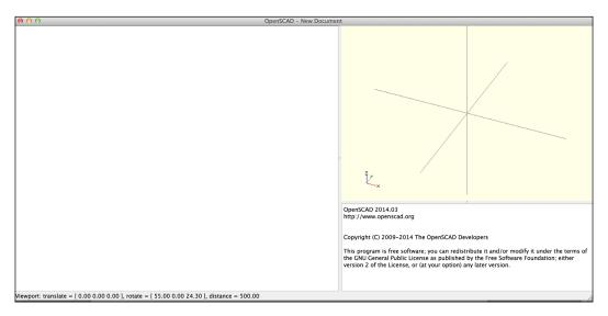
You can see that there are mainly three parts in the OpenSCAD window. There is some space for code on the left, a 3D view of the object on the right, and a window in the bottom-right corner to print out information about the project.
