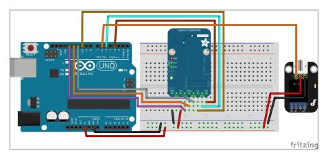
Note that this schematic only displays the connections for one relay module. Let's first see how to connect a single relay module. To get started on the hardware connection, first place the different components next to each other and plug the CC3000 module on the breadboard. We are first going to take care of the power supply part. Connect the ground (GND) pin of the Arduino board to the GND pin of the CC3000 board. Then, connect the Arduino Uno board 5V pin to the Vin pin of the CC3000 board.
