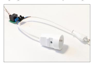
A relay module basically has three output pins: COM (for common pin), NC (for normally closed), and NO (for normally open). What we want is to have the COM pin connected directly to one pin of the power plug, NC not connected, and NO connected to another pin of the power plug.
