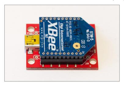
Now that this is done, you can power up everything by connecting the Arduino board and explorer module to your computer via USB cables.
