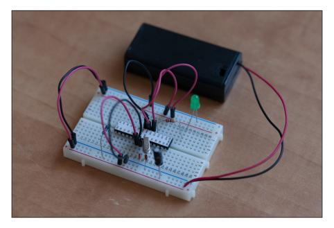
We can now test the project, just to see if it is working correctly. To do so, we are going to make the LED flash with the **Blink** sketch that comes with the Arduino IDE.
