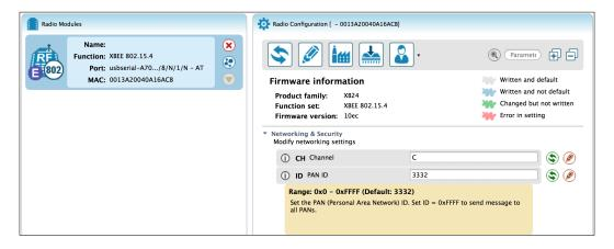
You will then be able to change the PAN ID of your device. To configure all the modules in your network, just repeat the procedure for each XBee module.
