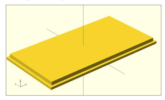
When your design is finished, you will have to export it to a special file format so that it can be 3D printed. To do so, go to **File** | **Export** and export the file as STL, which is the format required by many 3D printers and 3D-printing manufacturers.
