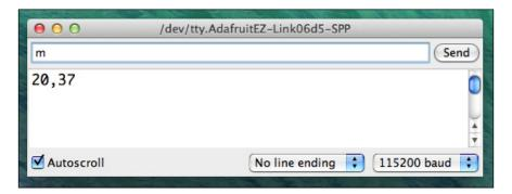
If you can see the measurements being printed out on the serial monitor, it means that the sensor is working correctly. It also means that the project is responding as expected when it receives the signal to measure data.
