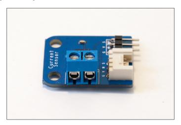
You can see in the preceding image that the board has three pins: G for ground, V for VCC, and S for signal, which will deliver the output voltage that is proportional to the measured current.
