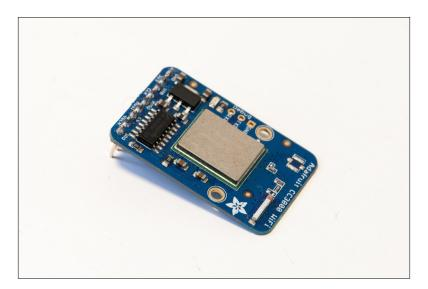
Again, you have quite a lot of options when choosing this board. You can pick one from any of your favorite manufacturers. It just needs to integrate the CC3000 Wi-Fi chip and be compatible with 5V voltage levels (which is the case for most CC3000 boards). You can also use an Arduino shield that integrates the CC3000 chip, like the one from Adafruit.
