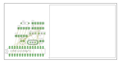
From here, your job is to place the different components (that we chose in the previous step when creating the schematic) on the board, arrange them as you want, and route the board. Routing refers to connecting the different components together on the board using copper traces. This can be done automatically by using the autorouting functionality of EAGLE. You can see that EAGLE already indicates which components are connected together by displaying thin lines between their pins.
