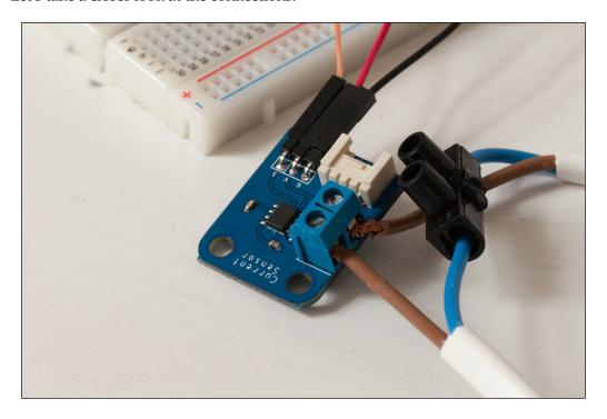
The idea is to have two wires of the power cables connected together (via a black connector, as shown in the preceding image), and the other two connected to the current sensor board. This way, the current sensor will sense the current going into the wires. The following schematic diagram illustrates the different connections for this part:
