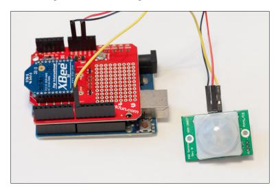
You will also need to set a jumper correctly on the board so we can upload a sketch. On the XBee shield, you have a little switch close to the XBee module to choose between the XBee module being connected directly to the Arduino board serial interface (which means you can't upload any sketches anymore) or leaving it disconnected. As we need to upload the Arduino sketch first, you need to put this switch to **DLINE**, as shown in this image:
