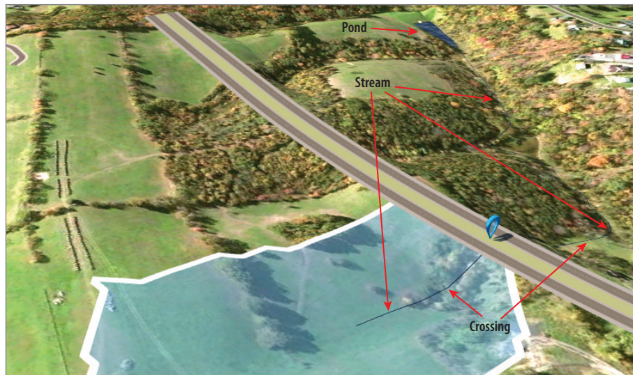
FIGURE 2.19 An existing stream crossing beneath the Bimsville Bypass
