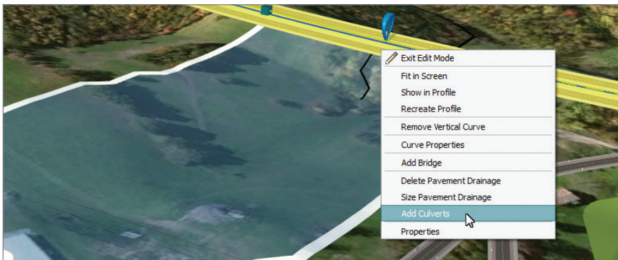
FIGURE 2.18 The Add Culverts command
