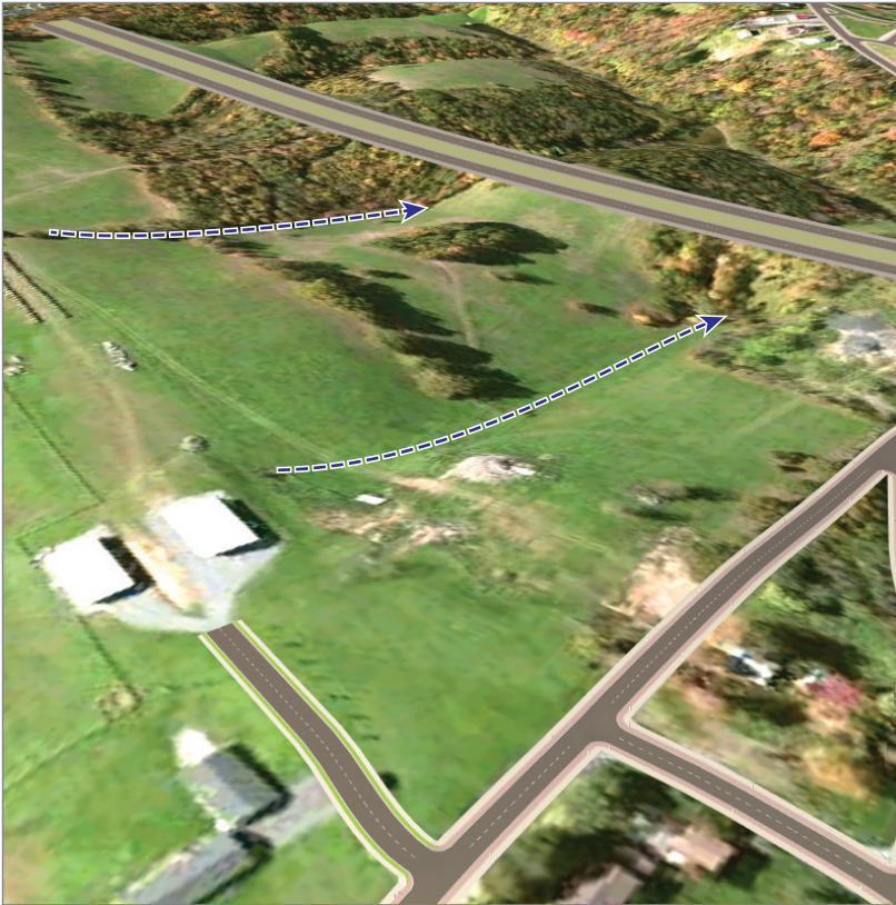
FIGURE 2.9 A design road is obstructing the flow of water.
