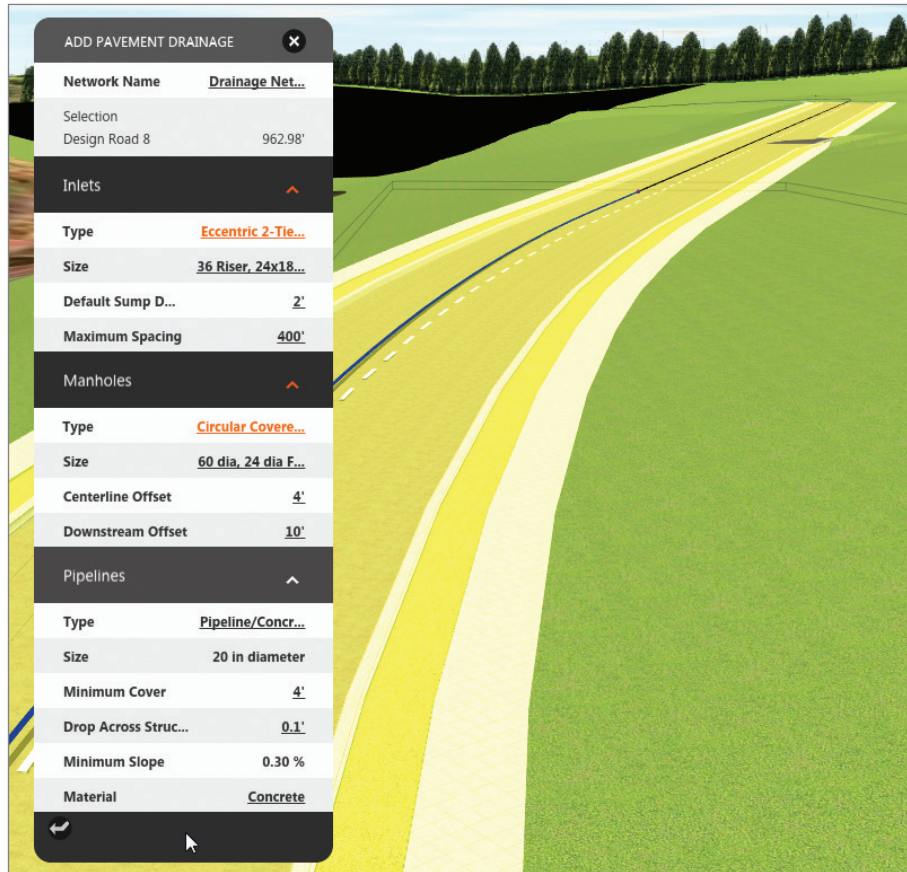
FIGURE 3.1 The Add Pavement Drainage asset card
