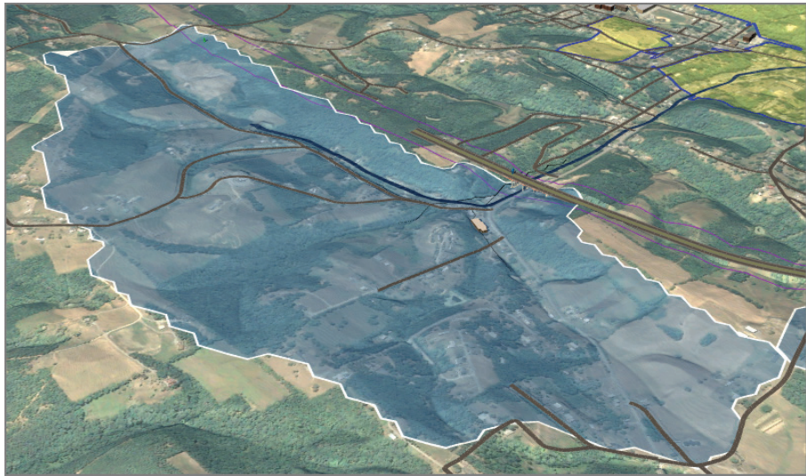
FIGURE 1.1 The blue shaded area is a watershed contributing flow under the bridge shown near the center of the image.
