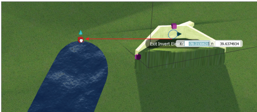
FIGURE 2.27 Relocating the end of a culvert
