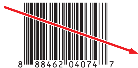
Figure 1.3 A laser needs to cross all bars of a 1D barcode for scanning
