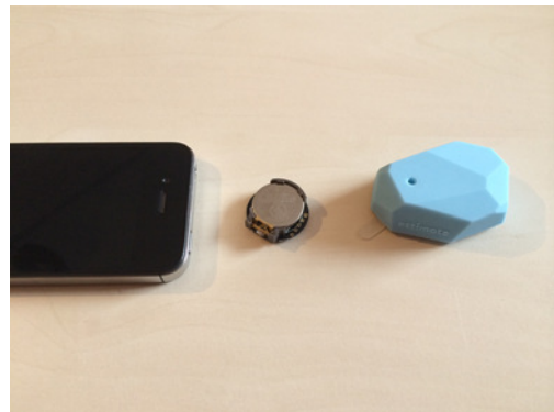
Figure 7.9 Two hardware iBeacons compared to iPhone
