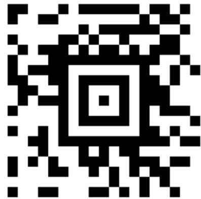
Figure 1.14 An example of an Aztec Code
