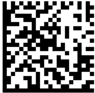
Figure 1.15 An example of a Data Matrix Code
