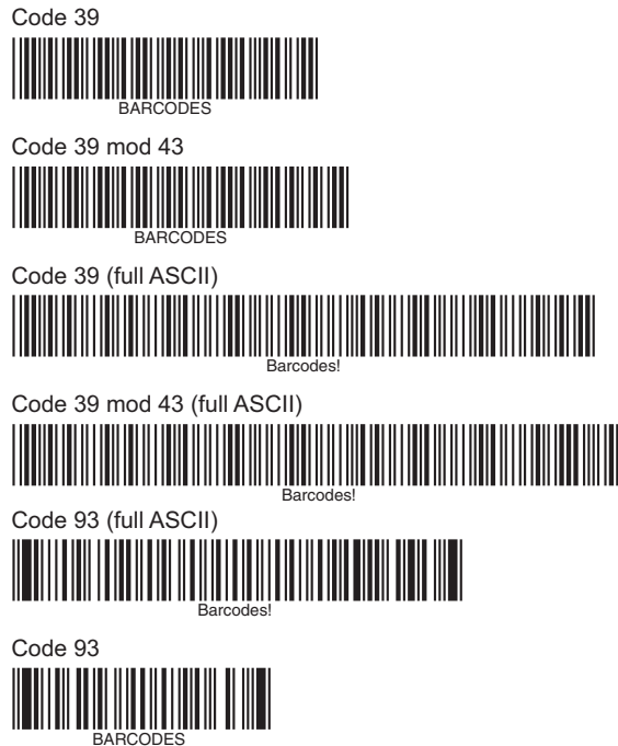
Figure 1.8 Code 93 is an optimized version of Code 39, developed by the same company, Intermec.
