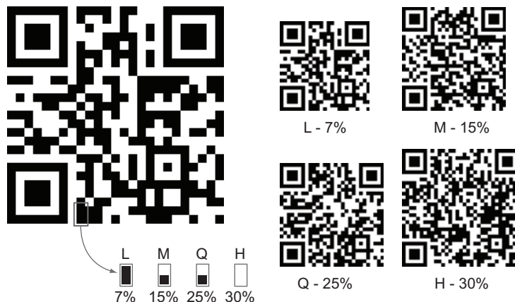
Figure 5.1 QR Code error-correction levels
