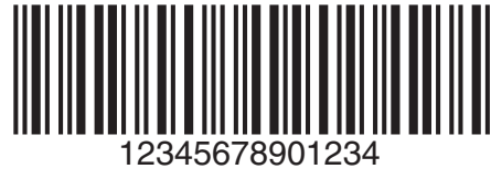
Figure 1.10 An example of an Interleaved 2 of 5 code
