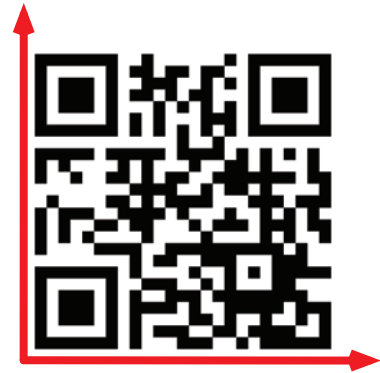
Figure 1.4 A CCD camera can “see” the squares that make up a 2D barcode.
