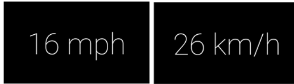
Figure 9-19. The digital speedometer Glassware creates a LiveCard that displays the current speed. By default, the speed is displayed in miles per hour (left). Users can toggle the display to use kilometers per hour (right)
