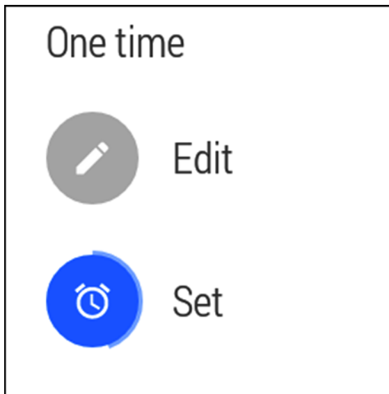
Figure 5-7. The native alarm app uses DelayedConfirmationView to give the user a few seconds to change or cancel the alarm
