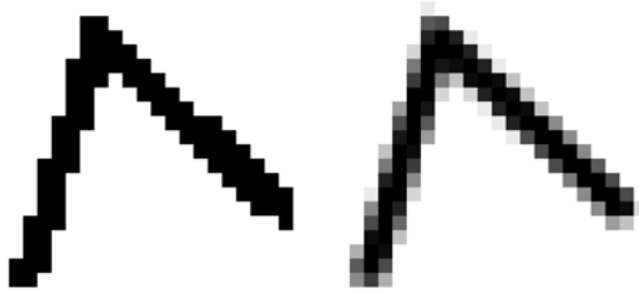
Figure 7-2. A bent line drawn with antialiasing disabled (left) and enabled (right)
