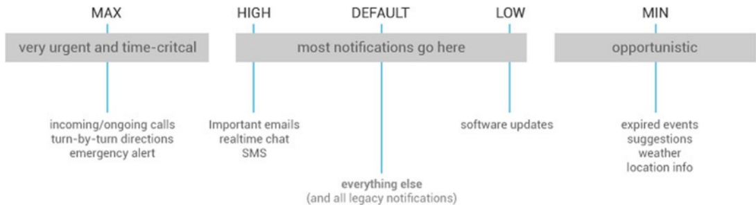
Figure 2-4. The significance of each value of notification priority. Diagram taken from the notification design documentation ( http://developer.android.com/design/patterns/notifications.html )
