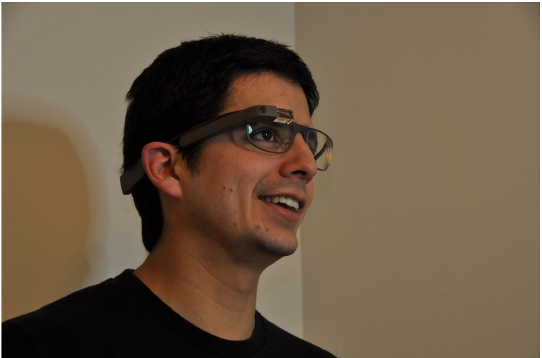
Figure 1-4. The screen of Glass sits above the user's eye
