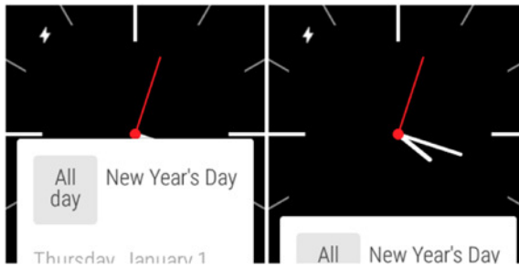
Figure 7-8. The card peek mode can take a value of WatchFaceStyle.PEEK_MODE_VARIABLE (left) and WatchFaceStyle.PEEK_MODE_SHORT (right)
