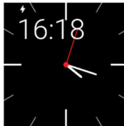
Figure 7-14. Showing the system UI time overlays the time in digital representation on top of the watch face
