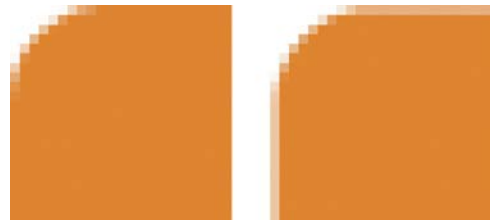
FIGURE 10.11 The left side shows what a graphic should look like when your pixels are aligned properly—it will come out looking crisp. The right side, when viewed at 100 percent, will look fuzzy.
