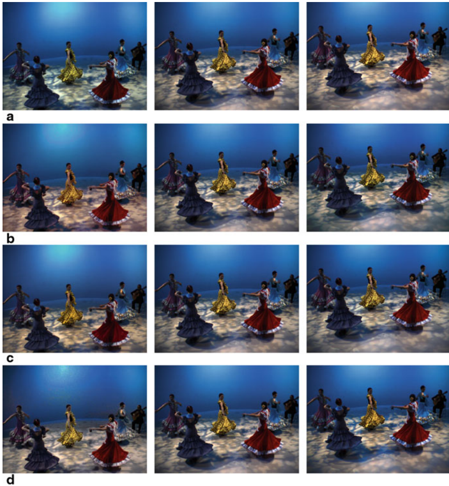
Fig. 10.3 Visual effect of color correction methods on the Flamenco2 test sequence ( left : view 1, middle : view 3, and right : view 5). Comparison between a without correction, b HM method [9], c Fezza et al. [11], and d Pitié et al. [44]
