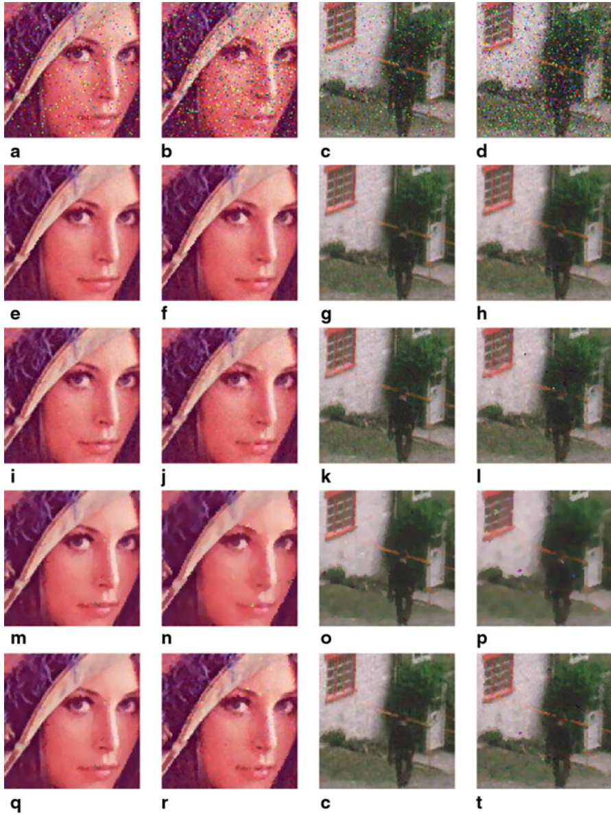
Fig. 4.8 Outputs for filter performance comparison of noise model IV. a, b Lenna corrupted with \alpha = 0.7 and \alpha = 0.5 . c, d Goldhill corrupted with \alpha = 0.7 and \alpha = 0.5 . e-h Output of INR. i-l Output of QRVF; m-p Output of SFRF. q-t Output of RWVMF
