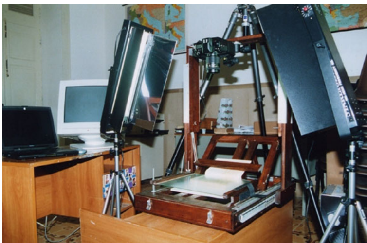
Fig. 7.9 Experimental setup for grabbing digital images
