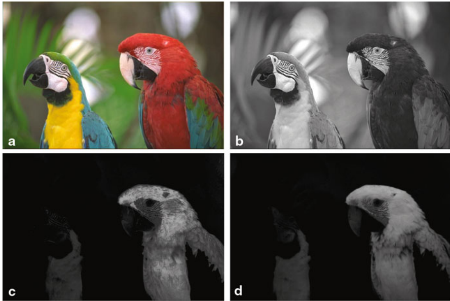
Fig. 2.7 Compare ratio image and difference image. a Original image, b Green plane, c R/G ratio image, d R - G difference image
