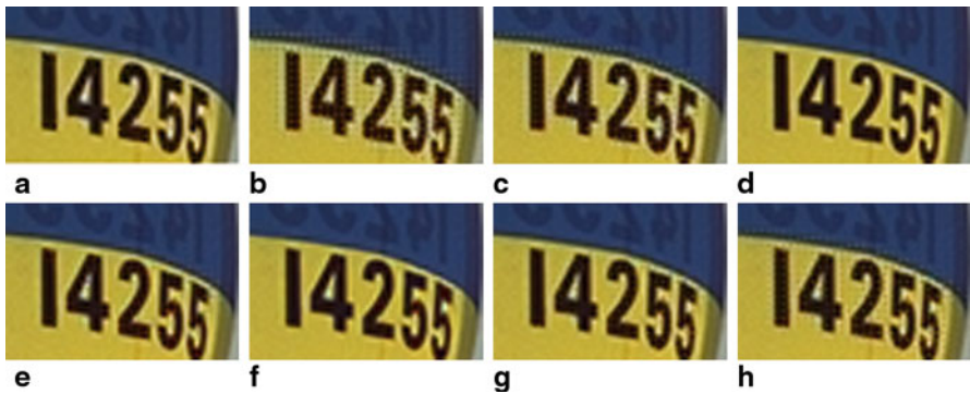
Fig. 2.20 Original and demosaiced results of a cropped region from test image 10. a original b HPHD-AI [59] c AHD [27] d DFAD [44] e LPA [52] f AP [24] g SA [33] h FD [7]
