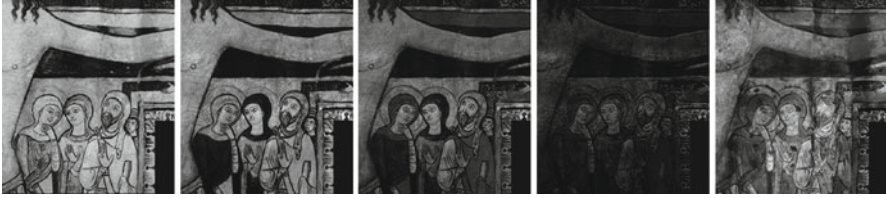
Fig. 7.32 From the left-hand side, multispectral images are shown, obtained, respectively, at the following wavelengths: 900 nm (IR), 700—450 nm (RGB), 400 nm (UV)
