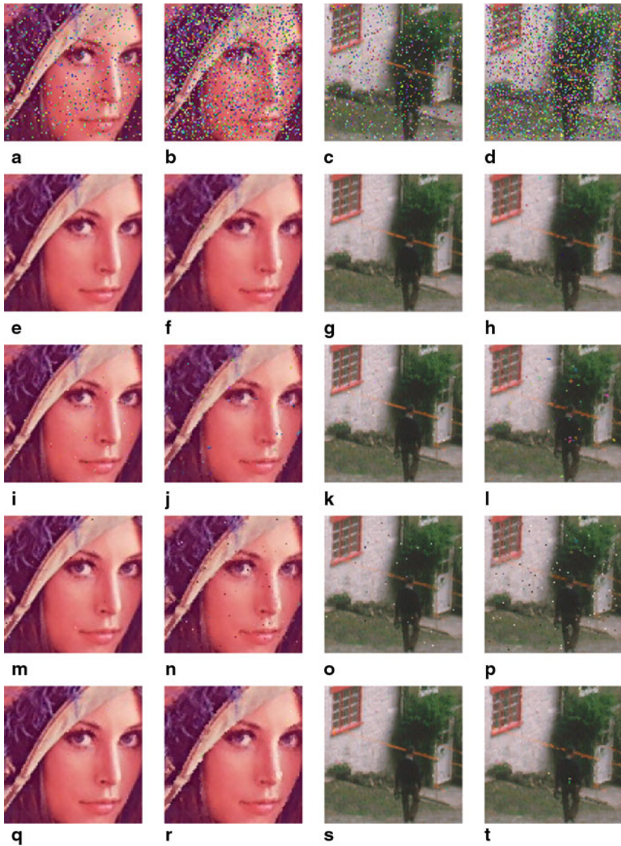
Fig. 4.6 Outputs for filter performance comparison of noise model II. a, b Lenna corrupted with p = 10\% and p = 30\% . c, d Goldhill corrupted with p = 10\% and p = 30\% . e-h Output of FPGF. i-l Output of FRF. m-p Output of IPGSVF. q-t Output of QRVF
