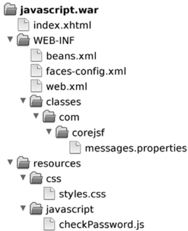
Figure 4-2 The JavaScript example directory structure
