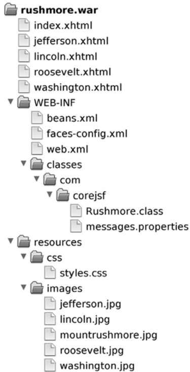
Figure 8-5 Directory structure for the Rushmore example
