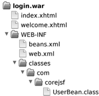
Figure 1-3 Directory structure of the sample WAR file
