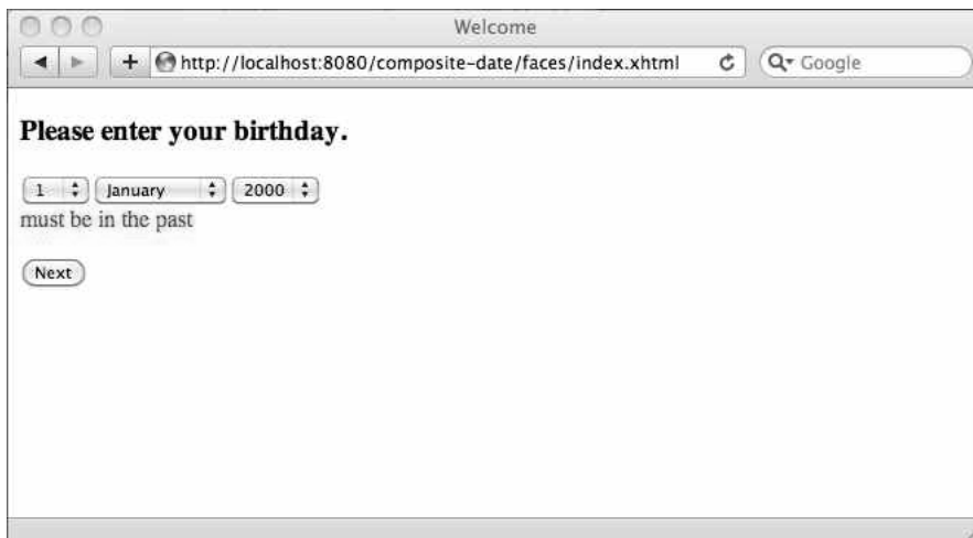
Figure 9–12 Trying to enter a date in the future is rejected with a validation error
