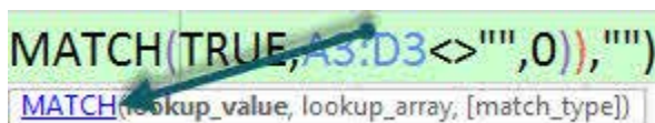
Figure 23.7 Clicking on the function name in the ScreenTip will open up the Help article for the function.
