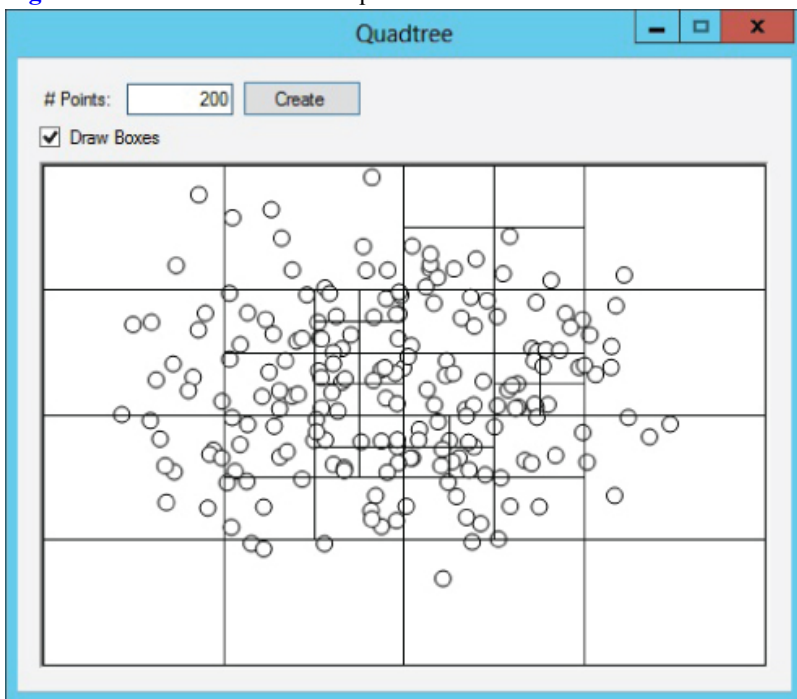
Figure 10.19 Each box shows a quadtree node's area.
