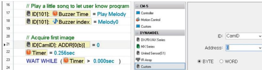
Fig. 9.12 Line 21—CUSTOM Command to capture and process a new video frame with HaViMo2
