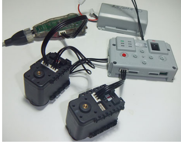
Fig. 4.4 Typical setup for Dynamixel firmware update using a CM-530 and two AX-12As
