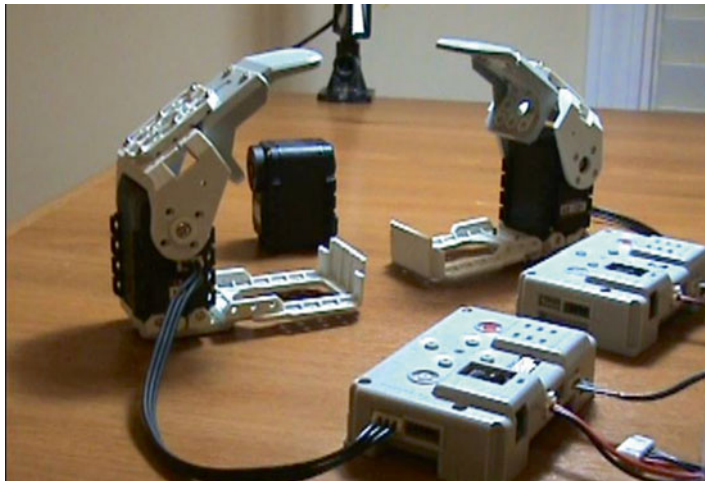
Fig. 8.6 Leader and follower grippers using 1-to-1 ZigBee
