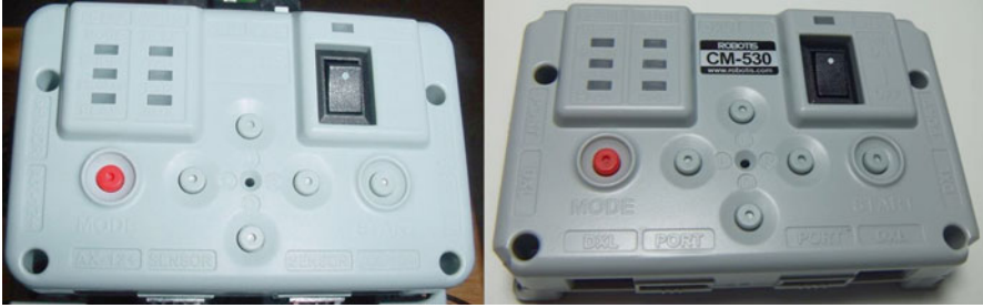
Fig. 2.9 CM-510 (discontinued) and CM-530 controllers
