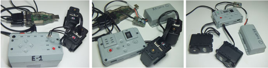
Fig. 4.10 Demonstration setups for TASK “comparative study” (left to right—CM-5, CM-510 and CM-530)
