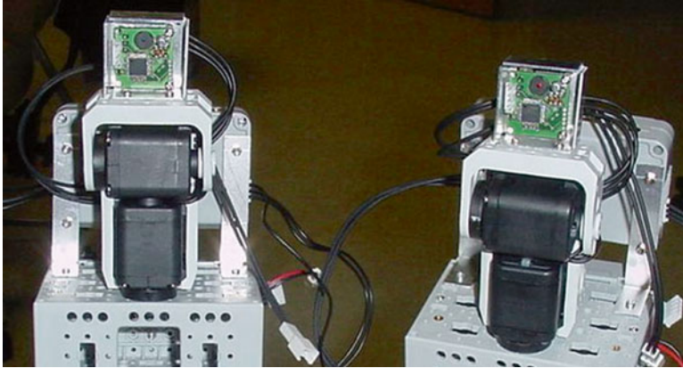
Fig. 3.29 HaViMo 2.0 video cameras mounted on PREMIUM BiPed
