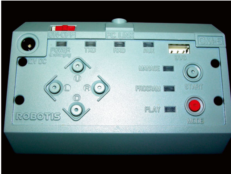
Fig. 2.7 CM-5 Controller (discontinued)
