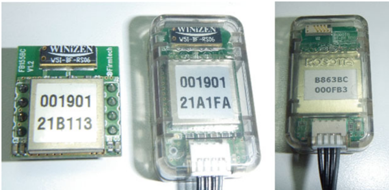
Fig. 3.10 BlueTooth communication devices BT-100/110A and BT-210
