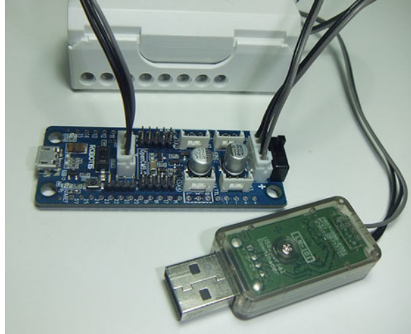
Fig. 4.9 Typical setup for controller firmware update for an OpenCM-9.04-C
