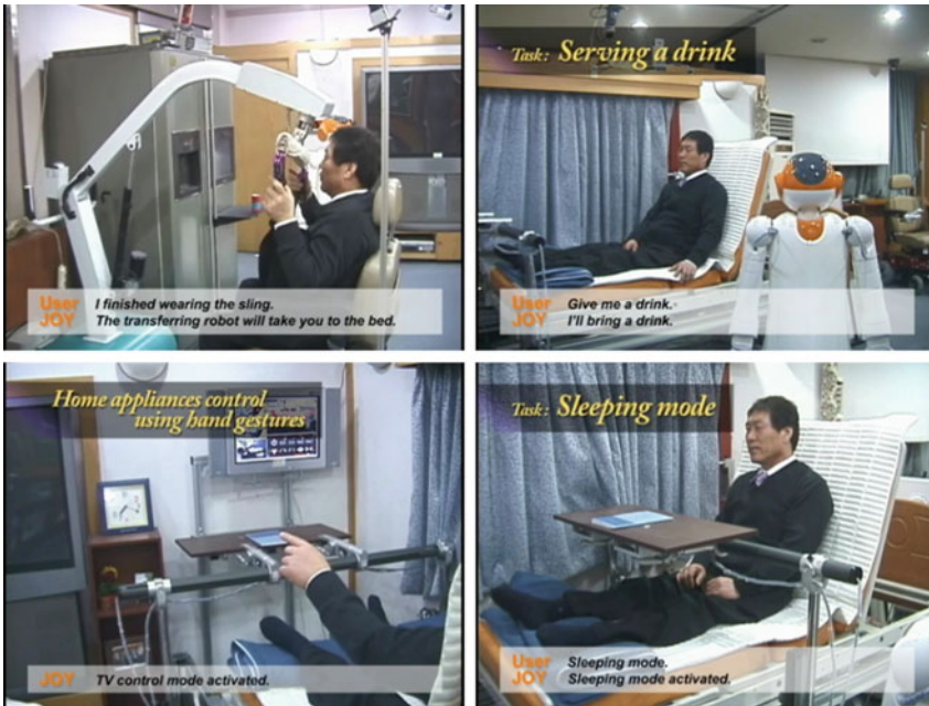
Fig. 2 KAIST's intelligent sweet home scenario. Multiple agents interact to provide a user with disabled lower-limbs a variety of proactive services, which consists of multiple low-level commands carried out by a transferring robot (shown in the upper left), a steward robot (shown in the upper right), a hand gesture-based soft remote control system (shown in the lower left), and an intelligent bed with a robotic arm (shown in the lower right)
