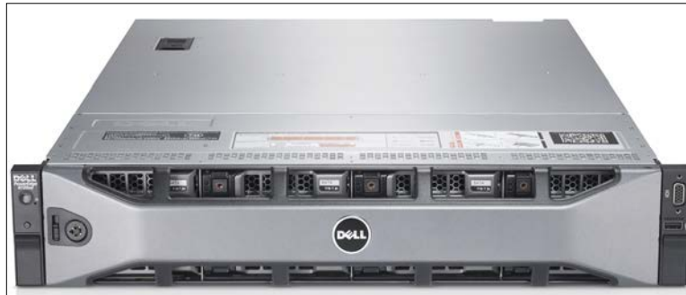
Server hardware used as a VSAN node
