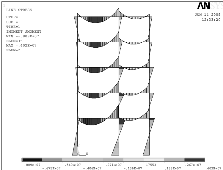
Fig. 4.17 Moment curve for the 2-bay and 5-storey planar frame structure (In Case 2)
