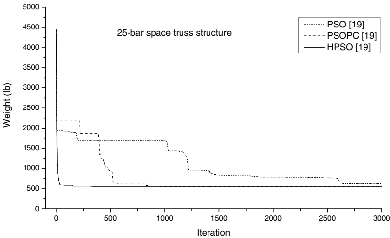
Fig. 3.11 Convergence rates of the three algorithms for the 25-bar spatial truss structure
