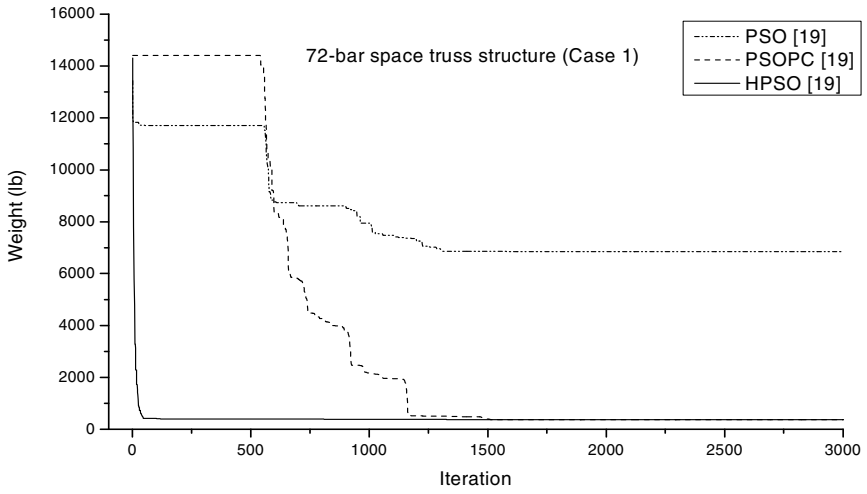
Fig. 3.14 Convergence rates of the three algorithms for the 72-bar spatial truss structure (Case 1)
