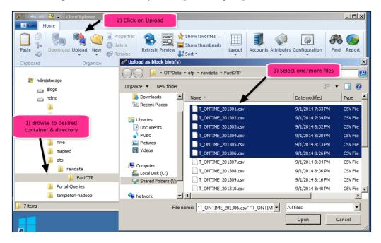
With the preceding steps, we have uploaded the six .csv files to Azure Blob storage using CloudXplorer.
