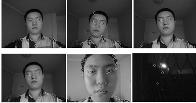
FIGURE 8.8 Image showing results from step 1 to find the circular-shaped objects.
