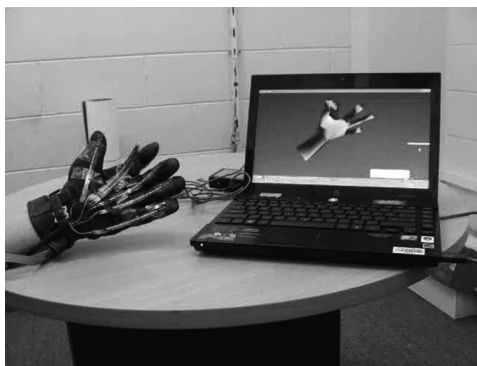
FIGURE 2.3 Smart glove for controlling the virtual hand developed at Biosignals Lab, RMIT University, Melbourne, Australia.
