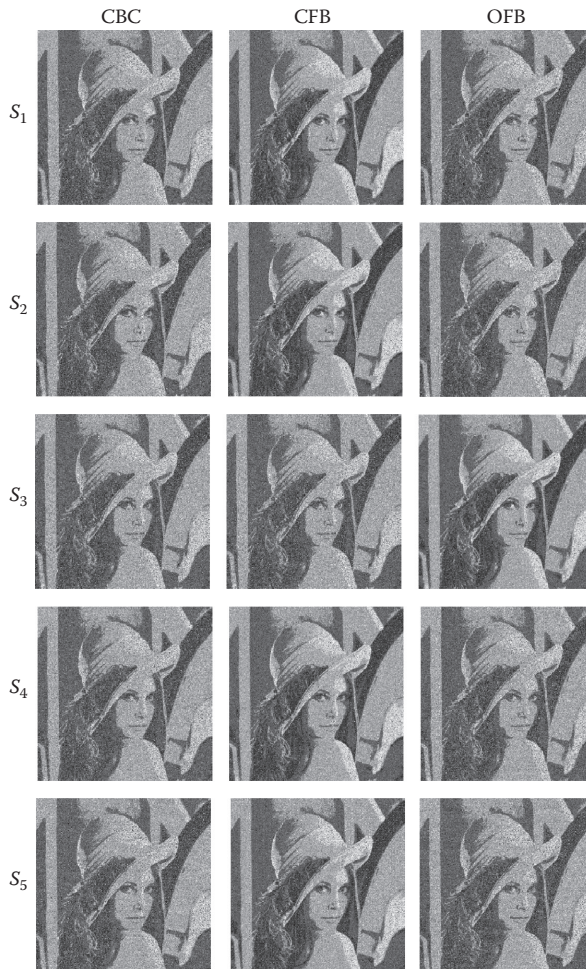
Figure 5.6 Decrypted images using the chaotic algorithm with different modes of operation and different block sizes at SNR = 5 dB.
