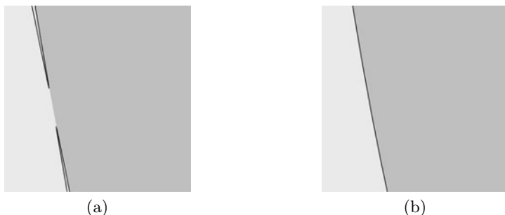
Fig. 6 (a) Result of fitting a nearly-straight boundary curve with a quadratic equation. (b) Result of applying perturbed technique to the same curve.
