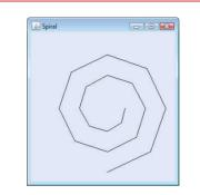
Fig. 13.33 | Spiral drawn using method drawPolyline.
