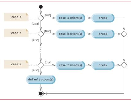
**Fig. 5.10** | switch multiple-selection statement UML activity diagram with break statements.
