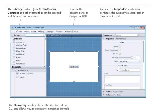
Fig. 25.7 | JavaFX Scene Builder displaying the default GUI in Welcome.fxml.
