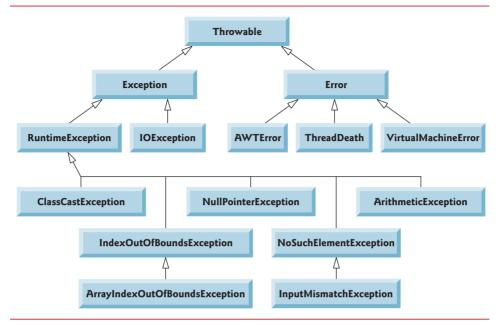
Fig. 11.4 | Portion of class Throwable's inheritance hierarchy.
