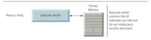
**Fig. 1.9** Typical Java development environment—verification phase.
