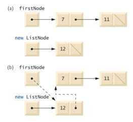
**Fig. 21.6** | Graphical representation of operation insertAtFront.
