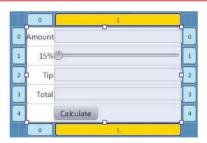
Fig. 25.14 | GridPane with columns sized to fit their contents.
