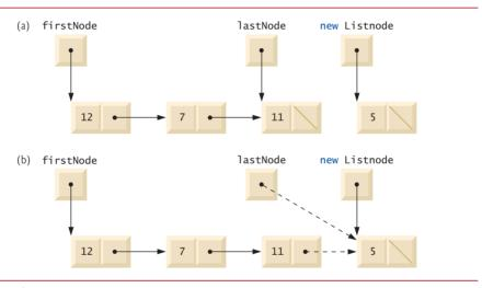
Fig. 21.7 | Graphical representation of operation insertAtBack.
