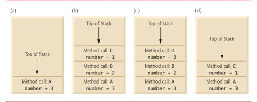
**Fig. 18.8** Method calls on the program-execution stack.
