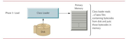
**Fig. 1.8** Typical Java development environment—loading phase.
