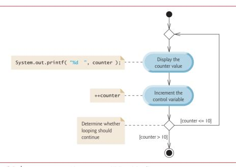
**Fig. 5.8** do...while repetition statement UML activity diagram.
