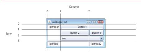
Fig. 22.18 Designing a GUI that will use GridBagLayout.
