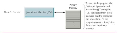
Fig. 1.10 | Typical Java development environment—execution phase.
