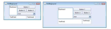
**Fig. 22.20** | GridBagLayout with the weights set to zero.
