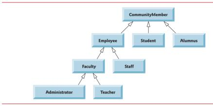
Fig. 9.2 | Inheritance hierarchy UML class diagram for university CommunityMembers.
