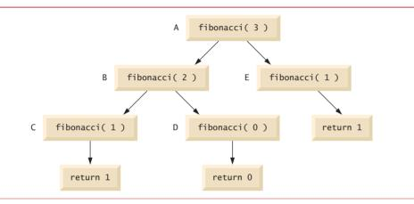
**Fig. 18.7** Method calls made within the call fibonacci (3).
