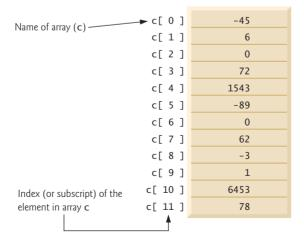
Fig. 7.1 | A 12-element array.
