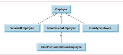
Fig. 10.2 | Employee hierarchy UML class diagram.
