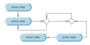
**Fig. 5.26** "Unstructured" activity diagram.
