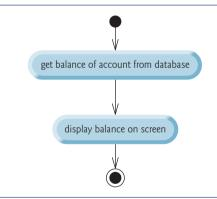
Fig. 12.14 Activity diagram for a BalanceInquiry object.
