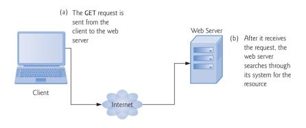
**Fig. 29.1** Client interacting with the web server. *Step 1:* The GET request.
