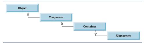
**Fig. 14.5** Common superclasses of the lightweight Swing components.
