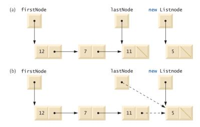
Fig. 22.7 | Graphical representation of operation insertAtBack.
