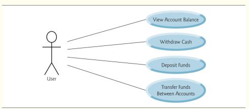
**Fig. 12.26** Use case diagram for a modified version of our ATM system that also allows users to transfer money between accounts.
