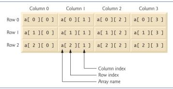
**Fig. 7.16** Two-dimensional array with three rows and four columns.
