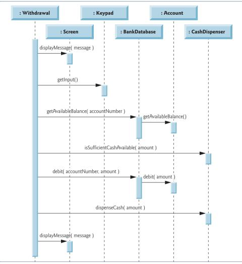
Fig. 12.25 | Sequence diagram that models a Withdrawal executing.
