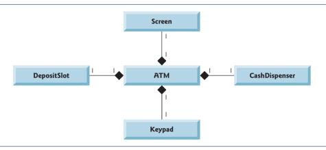
Fig. 12.9 | Class diagram showing composition relationships.
