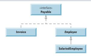
Fig. 10.10 | Payable interface hierarchy UML class diagram.
