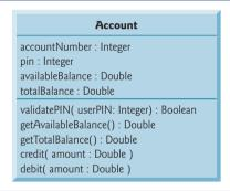
Fig. 12.19 | Class Account with operation parameters.
