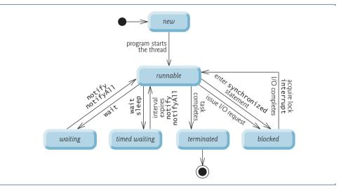
Fig. 26.1 Thread life-cycle UML state diagram.
