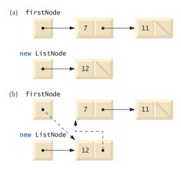
**Fig. 22.6** Graphical representation of operation insertAtFront.
