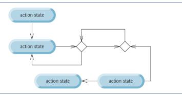
Fig. 5.25 | "Unstructured" activity diagram.
