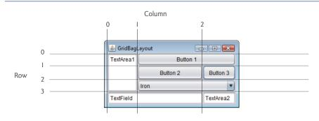
Fig. 25.18 Designing a GUI that will use GridBagLayout.
