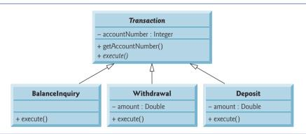
Fig. 13.8 | Class diagram modeling generalization of superclass Transaction and subclasses BalanceInquiry, Withdrawal and Deposit. Abstract class names (e.g., Transaction) and method names (e.g., execute in class Transaction) appear in italics.
