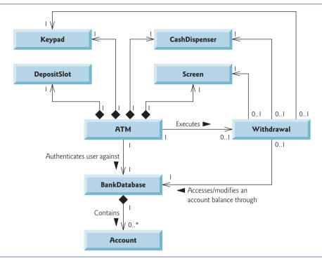
Fig. 13.2 | Class diagram with navigability arrows.
