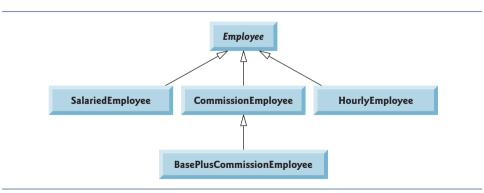
**Fig. 10.2** | Employee hierarchy UML class diagram.
