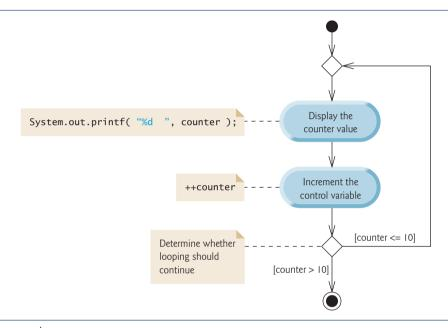
**Fig. 5.8** do...while repetition statement UML activity diagram.
