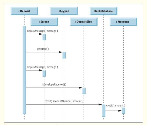
**Fig. 12.30** | Sequence diagram that models a Deposit executing.
