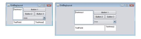
**Fig. 25.20** | GridBagLayout with the weights set to zero.
