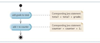
**Fig. 4.1** | Sequence structure activity diagram.
