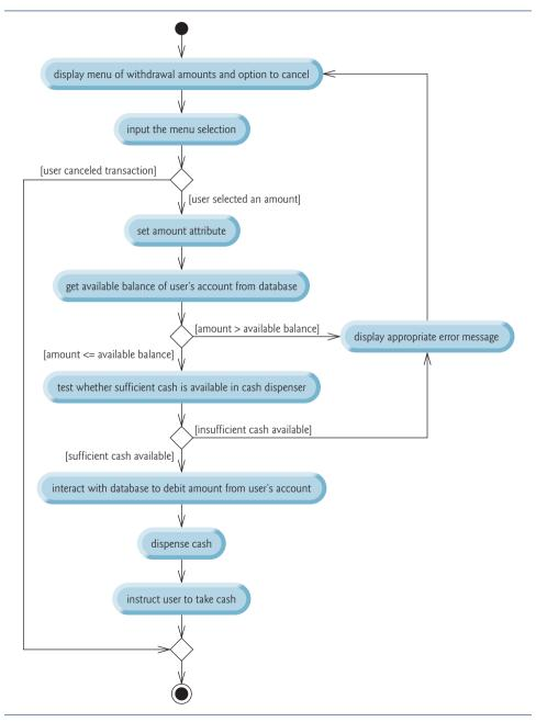
Fig. 12.15 | Activity diagram for a withdrawal transaction.
