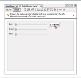
Fig. 1.5 | Positioning the first JTextField.
