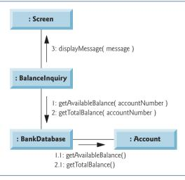
Fig. 12.24 | Communication diagram for executing a balance inquiry.
