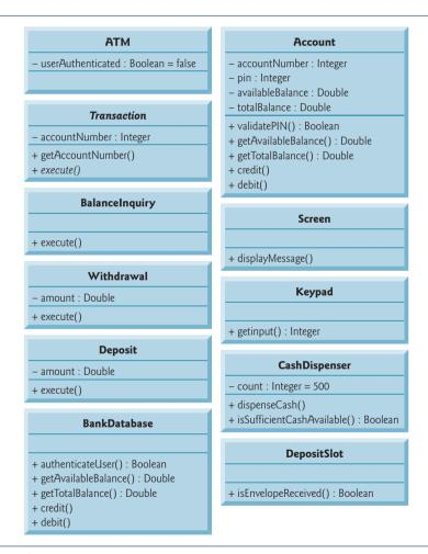
**Fig. 13.10** | Class diagram with attributes and operations (incorporating inheritance). The abstract class name Transaction and the abstract method name execute in class Transaction appear in italics.
