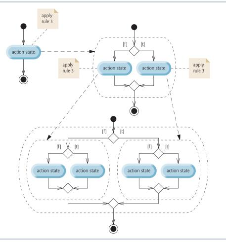
**Fig. 5.24** Repeatedly applying the Rule 3 of Fig. 5.21 to the simplest activity diagram.
