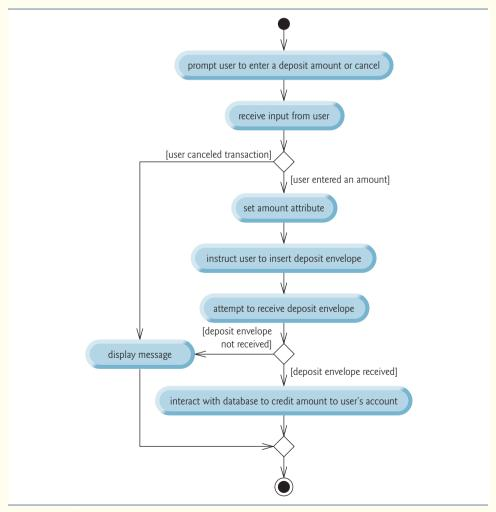
**Fig. 12.29** Activity diagram for a deposit transaction.
