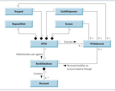
Fig. 12.10 | Class diagram for the ATM system model.
