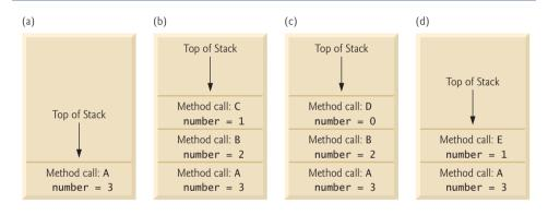
**Fig. 18.8** Method calls on the program-execution stack.
