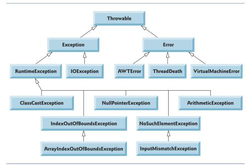
**Fig. 11.3** Portion of class Throwable's inheritance hierarchy.
