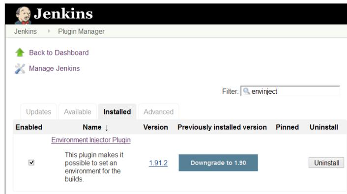
The EnvInject plugin provides the facility to have an isolated environment for different build jobs. The EnvInject plugin injects environment variables at node startup, before or after a SCM checkout for a run, as a build step for a run, and so on. Select **Inject environment variables to the build process** specific to the build job.
