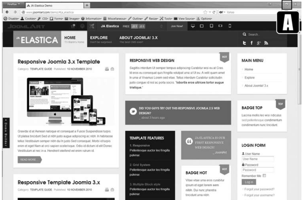
Figure 25-2 Set the [A] browser resizer to allow the edge of the browser window to be adjusted. This screenshot shows the browser window at full size on the desktop.
