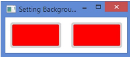
Figure 10-8. Two Panes having identical backgrounds set: one using CSS and one using Java objects
