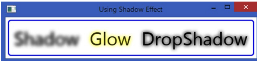
Figure 20-10. Applying a shadow to a Text node and creating Glow and DropShadow effects
