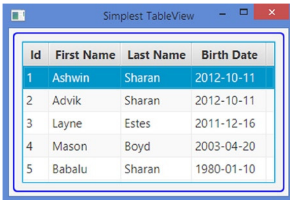
Figure 13-3. A window with a TableView that displays four columns and five rows
