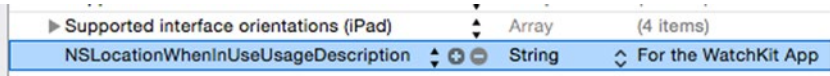
Figure 4-40. This key in the Info.plist file is required before a request for permission to use Core Location services can be made
