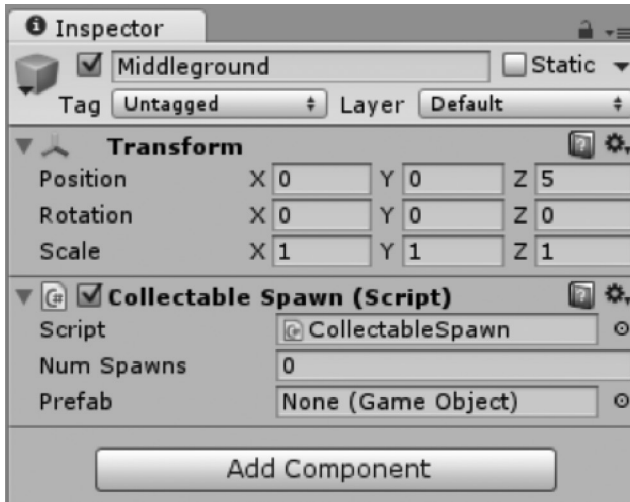
Figure 6.1 The CollectableSpawn script's numSpawns and prefab variables can be set from inside the Unity Inspector window. Similarly, whenever a variable is made public inside a script, it will automatically appear in the Unity Inspector and can be given a value there.
