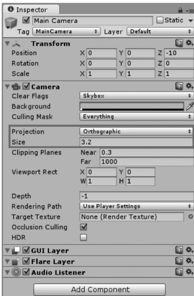
Figure 12.5 When using Unity in 2D mode, the main camera is set up for orthographic projection. Its size determines how large the camera's view is.
