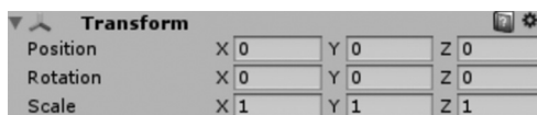
Figure 1.4 Every Unity object has a Transform component. The Position variable stores the coordinates of the object in the game world.
