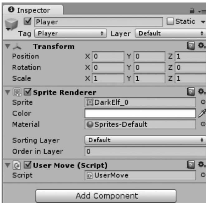
Figure 11.4 In the Unity scene, Luna is represented by the Player GameObject . This GameObject has Transform , SpriteRenderer , and script components.
