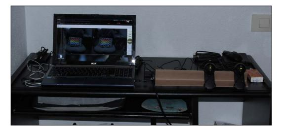
The calibration is done by the same <code>cameracalibrator.py</code> node used for monocular cameras. We pass the left-hand side and right-hand side cameras and images, so the tool knows that we are going to do stereo calibration. The following is the node in the launch file:
