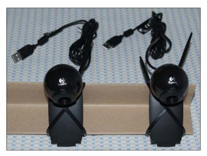
Now, connect the cameras to your USB slots. It is good practice to connect the left-hand side camera first and then the right-hand side one. This way, they are assigned to the /dev/video0 and /dev/video1 devices, or 1 and 2 if 0 was already taken. Alternatively, you can create a udev rule.
