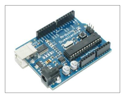
ROS can use this type of device with the rosserial package. Basically, Arduino is connected to the computer using a serial connection, and data is transmitted using this port. With rosserial, you can also use a lot of devices controlled by a serial connection, for example, GPS, servo controllers, and so on.
