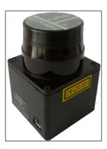
The Hokuyo URG-04lx model is a low-cost rangefinder commonly used in robotics. It has a very good resolution and is very easy to use. To start with, we are going to install the drivers for the laser:
