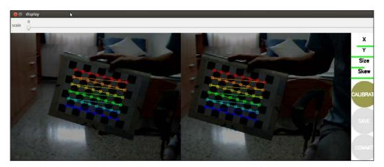
At the time the preceding image was taken, we showed enough views to start the calibration. Note that the calibration pattern must be detected by both cameras simultaneously to be included for the calibration optimization step. Depending on the setup, this may be quite tricky, so you should put the pattern at the appropriate distance from the camera. You can see the setup used for the calibration of this book in the next image:
