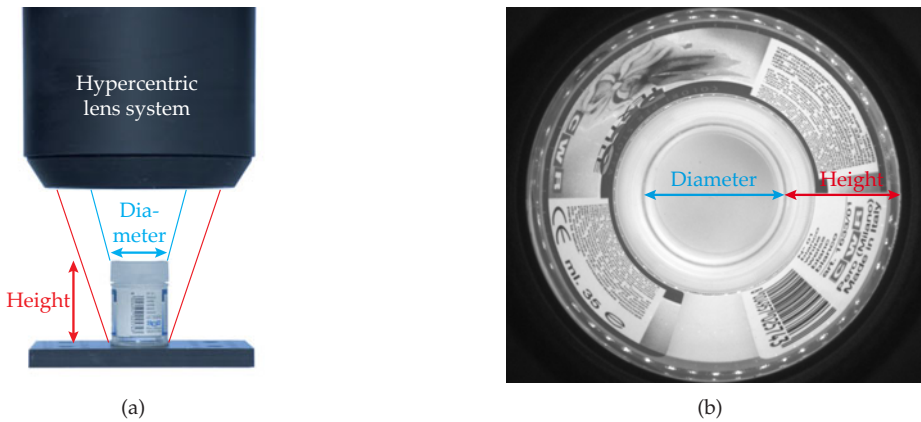
Figure 3.26. Hypercentric lens: (a) Imaging configuration; (b) Camera image. Both the cap and the outer surface of the cylindrically shaped test object are captured in the image, making it possible to measure, e.g., the object’s diameter and height (source: Opto Engineering srl).
