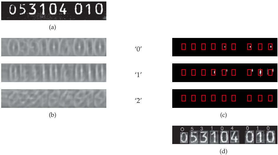
Figure 14.5. Optical character recognition using matched filters: (a) Gray-scale image g(\mathbf{x}) ; (b) Filtering results k_i(\mathbf{x}) for the characters '0', '1' and '2'; (c) Binary images, obtained by thresholding (b), superposed with the regions of interest (red rectangles); (d) Detection result.
