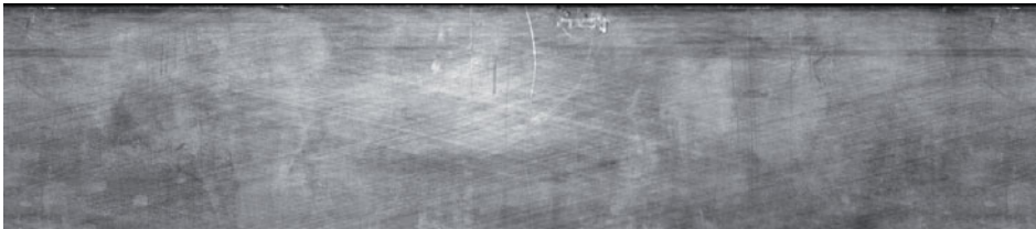
Figure 6.11. Image of a cylinder wall of a combustion engine, captured with a line-scan camera (source: Breitmeier Messtechnik GmbH).
