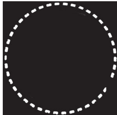
Figure 7.73. Automated visual inspection of a brake disk's ventilation channels: (a) Setup of the inspection system; (b) Sketch of a ventilated brake disk; (c) Resulting image (source: inspection GmbH).
