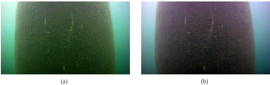
Figure 10.15. (a) Camera image of a pillar illuminated by daylight through the water surface. At this depth, the green and blue components of the spectrum of daylight are obviously already emphasized. The image degradations typical of participating media are clearly visible: color shifts, blurring, and a reduced contrast. (b) Result of image enhancement. By estimating a transmission map [13], the contrast, which had been lost due to the scattering caused by the turbidity, could be increased by means of a local histogram equalization.
