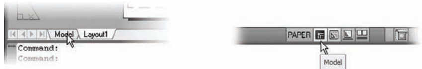
FIGURE 1.16 Click the Model tab (left) or the Quick View Layouts tool in the status bar (right).
