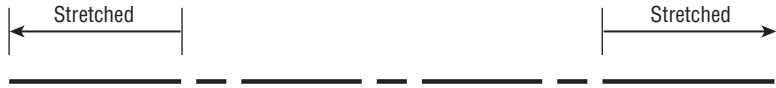
FIGURE 26.26 AutoCAD stretches the beginning and the end of the line as necessary.
