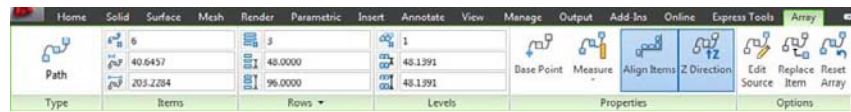
FIGURE 22.26 The Array tab appears and a new set of panels and options is displayed.
