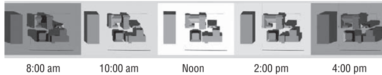
FIGURE 23.13 A series of simple renderings showing the way shadows fall from a set of buildings
