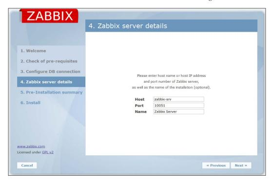
There is no check for the connection available on this page, so it is better to verify that it is possible to reach the Zabbix server from the network. In this form, it is necessary to fill **Host** (or IP address) of our Zabbix server. Since we are installing the infrastructure on three different servers, we need to specify all the parameters and verify that the Zabbix server port is available on the outside of the server.
