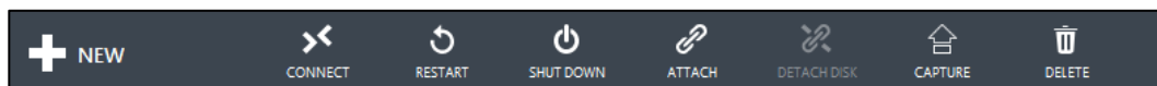
FIGURE 1-14 Actions for the selected resource, which in this case is a VM.
