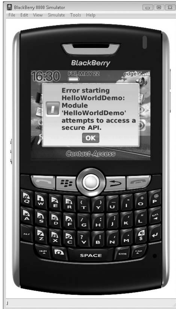
Figure 5-2 Error displayed when loading an unsigned application that uses RIM Controlled APIs.
