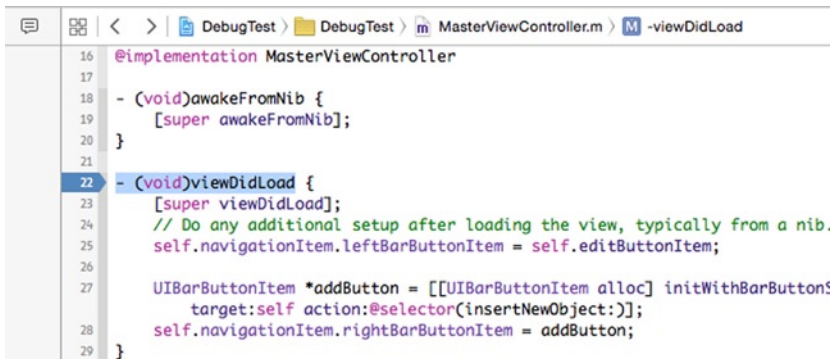
Figure 15-10. To the left of the editing pane is a column that usually shows line numbers. This is where you set breakpoints
