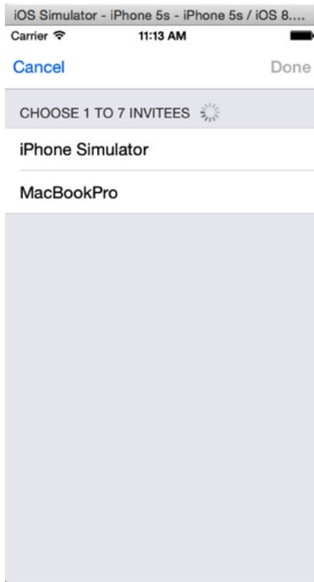
Figure 9-3. When another device within range starts a game, the two devices will show up in each other's peer picker dialog
