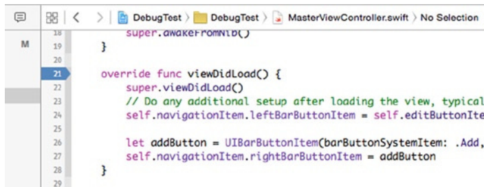
Figure 15-10. To the left of the editing pane is a column that usually shows line numbers. This is where you set breakpoints
