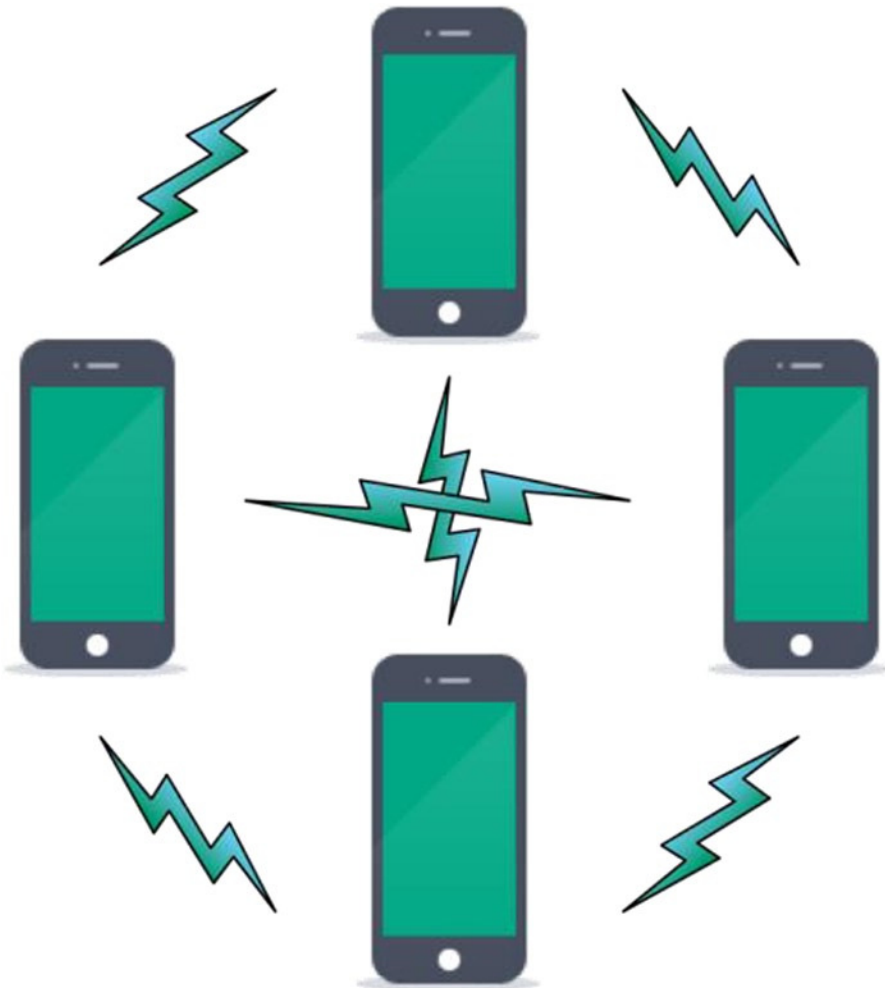
Figure 9-10. In the peer-to-peer model, peers can talk to each other directly and can continue to do so even in the absence of a server
