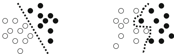
Fig. 13.17. A linearly separable two-class dataset (left) compared with a nonlinearly separable two-class dataset (right).
