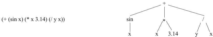
Fig. 7.1. Example S-expression (left) and corresponding syntax tree (right). The syntax tree decodes into the expression (\sin x) + (x * 3.14) + (y/x) , where x and y are predefined constants
