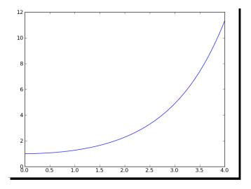
We plotted the modified Bessel function of the first kind 0th order with the NumPy  $\verb"i0"$  function.
