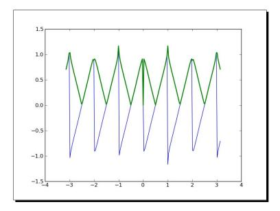
We drew a sawtooth wave using the sin function. The input values were assembled with linspace and the k values with the arange function. A triangle wave was derived from the sawtooth wave by taking the absolute value.
