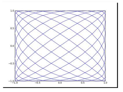
We plotted the Lissajous curve with the aforementioned parametric equations where A=B=1, a=9 and, b=8. We used the sin and linspace functions as well as the NumPy pi constant.
