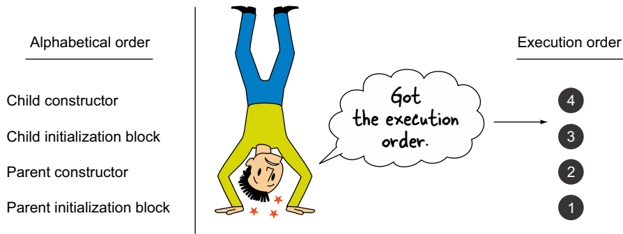
Figure 1.17 The order of execution of constructors and instance initializers in parent and child classes
