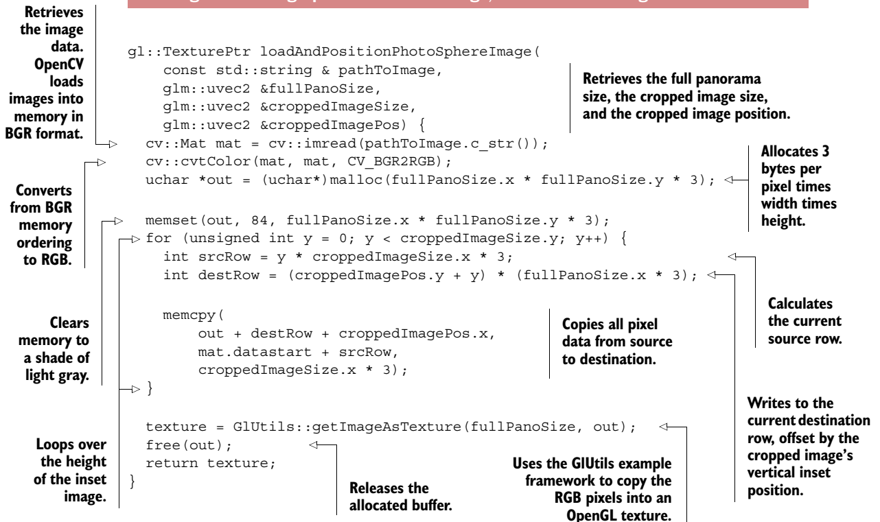
Listing 13.2 Using OpenCV to load an image, and then embedding it into a texture
