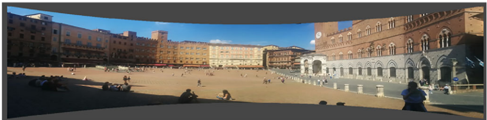
Figure 13.2 Cylindrical projection of the horizontal panorama. Note how the road (far right) has become straighter under projection.
