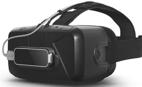
Figure 13.12 An Oculus Rift DK2 with the Leap Motion mounted on a removable bracket attached to the faceplate. The Leap can be popped out of the bracket holder and doesn't block the Rift's IR LEDs.
