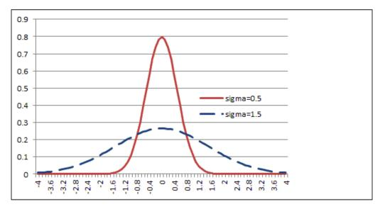
Pixels farther from the center have a lower weight, which makes the pixel-to-pixel transitions smoother. This contrasts with the flat mean filter where pixels far away can cause sudden changes in the current mean value. In terms of frequencies, this implies that the mean filter does not remove all the high frequency components.
