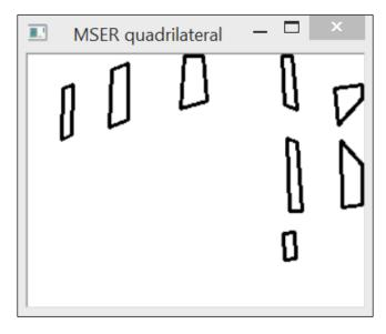
To detect rectangles, you can simply measure the angles between adjacent edges and reject the quadrilaterals that have angles that deviate too much from 90 degrees.
