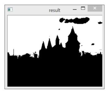
Here, a white pixel indicates a positive detection of the sought color, and black indicates negative.
