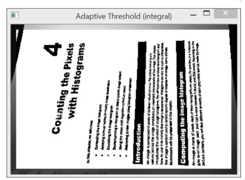
Clearly, this is a much better result than the one we got using a fixed threshold. Adaptive thresholding is a common image-processing technique. As such, it is also implemented in OpenCV as follows:
