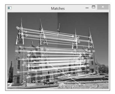
Interestingly, almost all these matches are correct, even if a few false matches remain; these accidently fell on the corresponding epipolar lines of the computed fundamental matrix.
