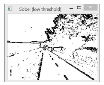
As can be seen, the edges that delineate the road are very well defined. However, because a permissive threshold was used, more edges than what is ideally needed are also detected. The role of the second threshold, then, is to define the edges that belong to all important contours. It should exclude all edges considered as outliers. For example, the Sobel edge map that corresponds to the high threshold used in our example is as follows:
