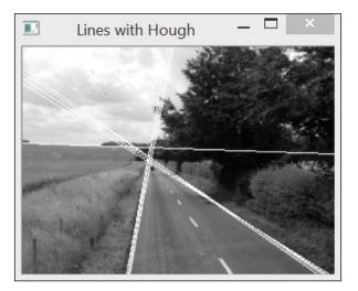
As can be seen, the Hough transform simply looks for an alignment of edge pixels across the image. This can potentially create some false detections due to incidental pixel alignments or multiple detections when several lines pass through the same alignment of pixels.
