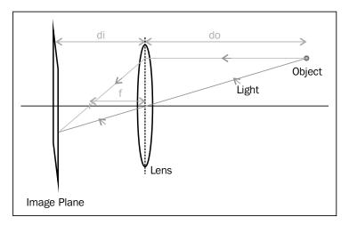
Here, **do** is the distance from the lens to the observed object, **di** is the distance from the lens to the image plane, and **f** is the focal length of the lens. These quantities are related by the so-called thin lens equation:
