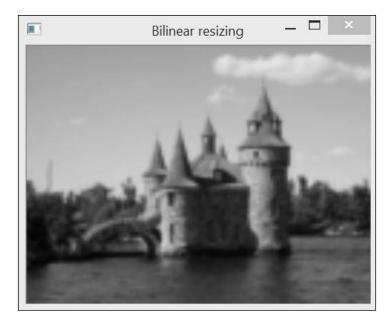
There also exist other approaches that can produce superior results. With **bicubic interpolation**, a neighborhood of 4x4 pixels is considered to perform the interpolation. However, since the approach uses more pixels and implies the computation of cubic terms, it is slower than bilinear interpolation.
