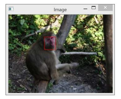
This time, we will describe this object by using the hue channel of the HSV color space. This means that we need to convert the image into an HSV one and then extract the hue channel and compute the 1D hue histogram of the defined ROI. Refer to the following code:
