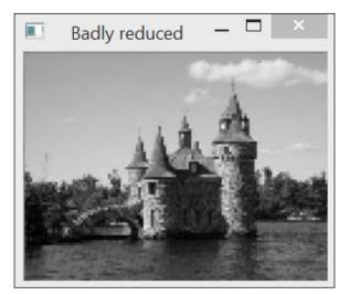
Clearly, one can see that the image quality has degraded. For example, the oblique edges of the castle's roof in the original image now appear as a staircase on the reduced image. Other jagged distortions are also visible on the textured parts of the image (the brick walls, for instance).
