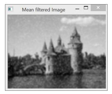
Clearly, the noisy pixels shifted the mean value of neighboring pixels. As a result, the noise is still visible even if it has been blurred by the mean filter.
