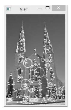
However, since the computation of the feature point is based on floating-point kernels, SIFT is generally considered to be more accurate in terms of feature localization in regards to space and scale. For the same reason, it is also more computationally expensive, although this relative efficiency depends on each particular implementation.
