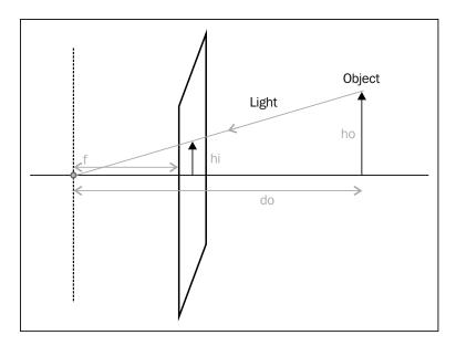
From this model, and using the law of similar triangles, we can easily derive the basic projective equation that relates a pictured object with its image:
