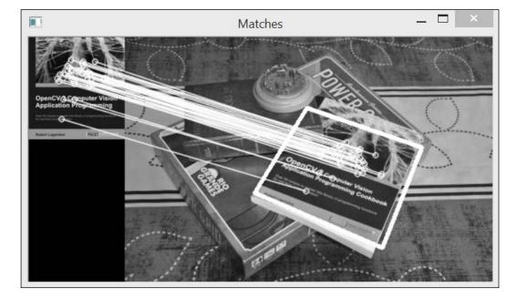
Using the  ${\tt cv::drawMatches}$  function, we display the results as follows:
