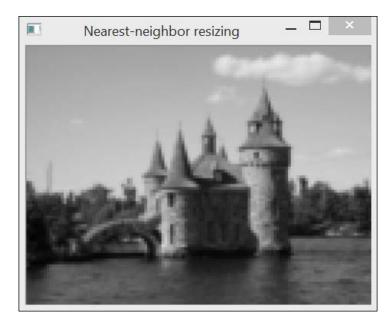
In this case, the interpolation corresponds to simply multiplying the size of each pixel by 3 (this is how we produced the images of the previous section). A better approach consists of interpolating a new pixel value by combining the values of several neighboring pixels. Hence, we can linearly interpolate a pixel value by considering the four pixels around it, as illustrated by the following figure:
