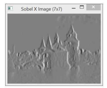
If you compare this image with the one shown earlier, it can be seen that many fine details have been removed, giving them more emphasis on the more significant edges. Note that we now have a band-pass filter, the higher frequencies being removed by the Gaussian filter and the lower frequencies being removed by the Sobel filter.
