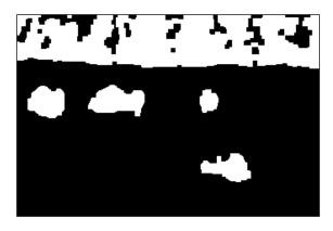
We obtained this image from a simple thresholding operation followed by the application of open and close morphological filters. This recipe will show you how to extract the objects of such images. More specifically, we will extract the **connected components**, that is, shapes made of a set of connected pixels in a binary image.
