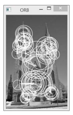
As can be seen, since the keypoints are independently detected on each pyramid layer, the detector tends to repeatedly detect the same feature point at different scales.
