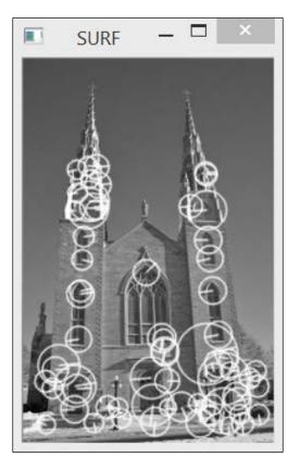
As explained in the previous recipe, the size of the keypoint circles resulting from the use of the DRAW\_RICH\_KEYPOINTS flag is proportional to the computed scale of each feature. The SURF algorithm also associates an orientation with each feature to make them invariant to rotations. This orientation is illustrated by a radial line inside each drawn circle.
