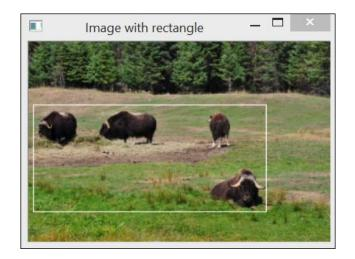
All the pixels outside this rectangle will then be marked as the background. In addition to the input image and its segmentation image, calling the cv::grabCut function requires the definition of two matrices, which will contain the models built by the algorithm as follows:
