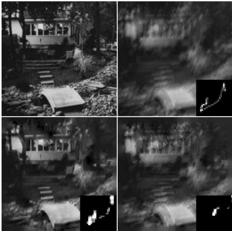
Fig. 4.8 Illustrating the performance of deconvolution: ground truth ( left upper ), blurred image ( right upper ), deconvolution result of [5] ( left lower ), and with a joint MAP estimator with edge reweighting ( right lower ). The blue kernel is depicted in the lower right area of the images (From Levin et al. [15], with kind permission)
