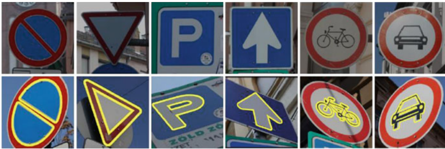
Fig. 2.10 Illustrating the aligning performance for some traffic signs. Top row : template shapes. Bottom row : matched templates in some query images visible as yellow overlays (© 2012 IEEE. Reprinted, with permission, from Domokos et al. [5])
