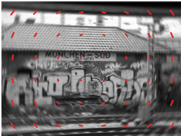
Fig. 4.10 Showing an example image with rotation blur together with some red paths defining the pixels being influenced by the same scene element when the camera is rotated around the z -axis (perpendicular to the image plane). Clearly, these paths depend on their position in the camera image. Blur caused by this rotation typically increases significantly in the edges of the image
