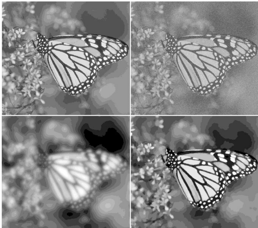
Fig. 4.2 Illustrating the performance of total variation regularization. Upper left : original image. Upper right : image with synthetically added noise. Lower left : denoising solution with Tikhonov regularization. Lower right : denoising solution with total variation (From Pock [20], with kind permission)
