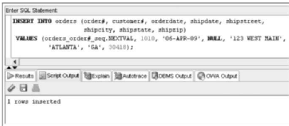
FIGURE 6-6 Inserting a row, using a sequence to provide a PRIMARY KEY value
