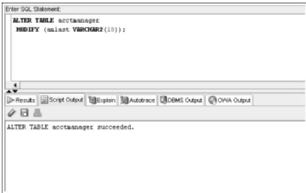
FIGURE 3-18 The ALTER TABLE ... MODIFY command to increase the column width
