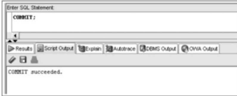
FIGURE 5-33 Command to save data changes permanently
