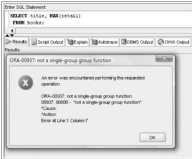
FIGURE 12-4 Flawed query: attempt to determine the book with the highest retail value
