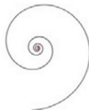
Figure 10-7. A spiral traced by a particle with decreasing velocity in a constant magnetic field
